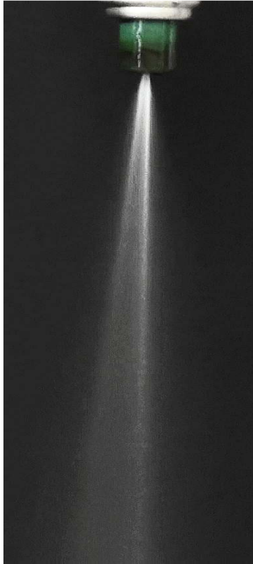
Figure 4.15 :Spray pattern for 4ms at 0.4Mpa
