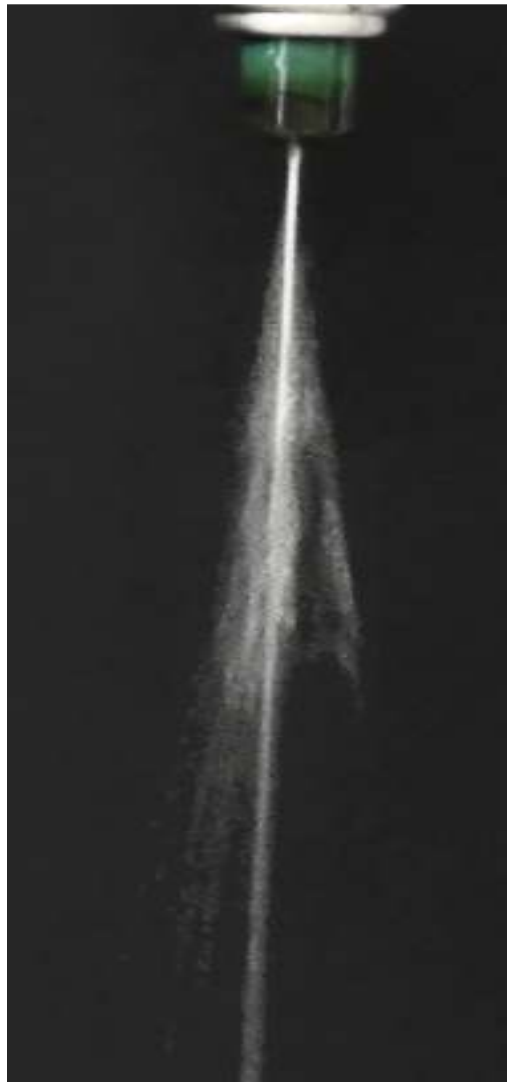
Figure 4.8 :Spray pattern for 1ms at 0.4Mpa
