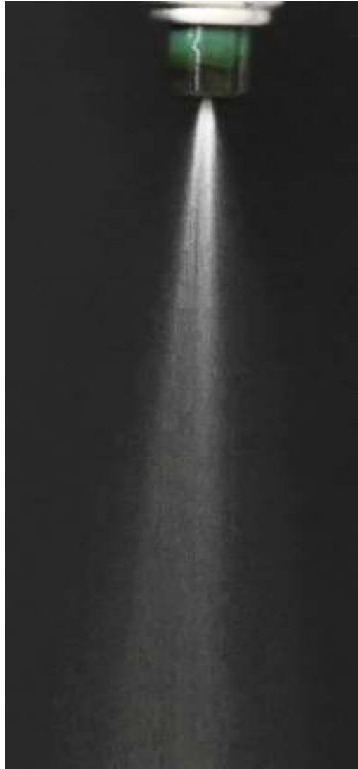
Figure 4.10 :Spray pattern for 3ms at 0.4Mpa
