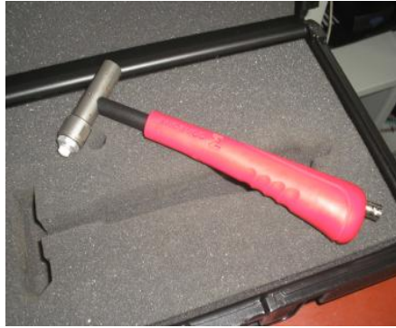
Figure 3.13: Impact hammer used in experiment
