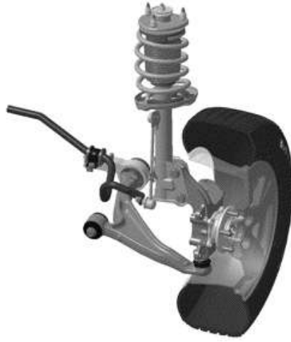
Figure 2.1: MacPherson strut suspension
