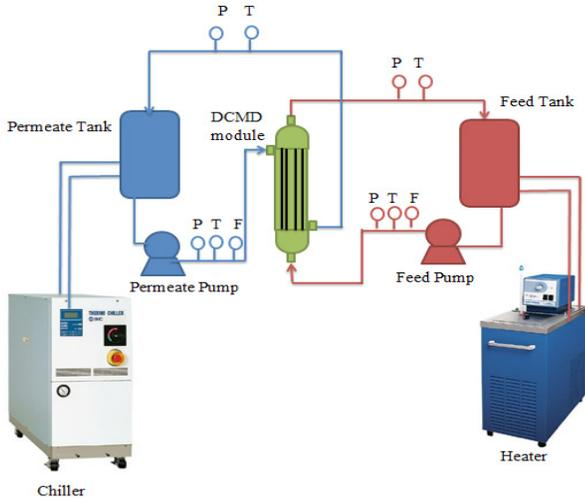
Figure 1. Schematic DCMD experimental setup.
