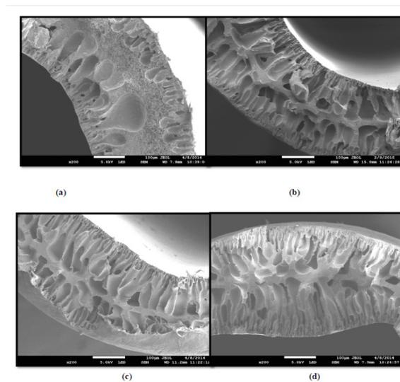
Figure 2. FESEM images of the Morphology for PVDF-co-HFP hollow fiber membranes prepared with: (a) 0% PVP, (b) 5% PVP, (c) 7% PVP, (d) 9% PVP.
