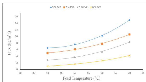
**Figure 3.** Flux as a function of feed temperature for (0.6 L/min) flow rate.
