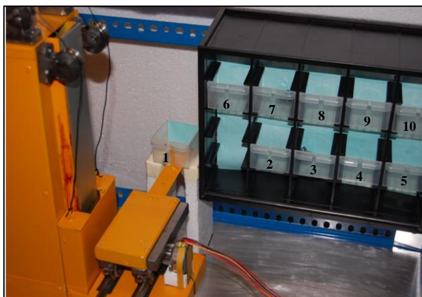
Figure 4.5e: Drawer picker move forward until arrive P/D station
