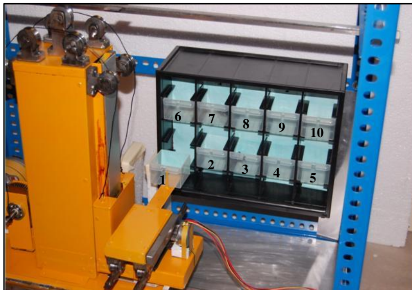
Figure 4.5c: Drawer picker move reversely with the drawer
