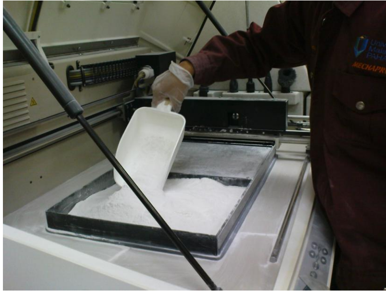
Figure 3.7: Filling the feed box with powder
