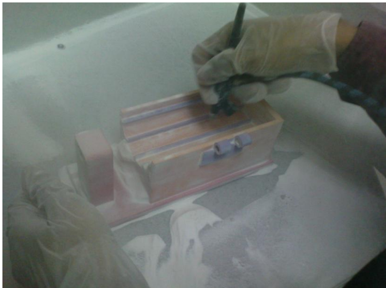
Figure 3.10: Fine depowder part
