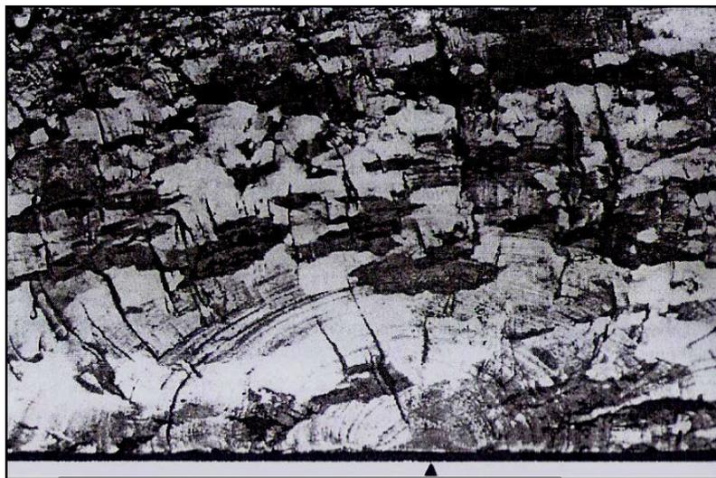
**Figure 2.26:** Fracture surface of a light metal compressor blade. The fatigue failure started at the lower surface (arrow).
