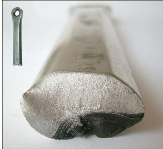
**Figure 2.6:** Crack growth due to fatigue
