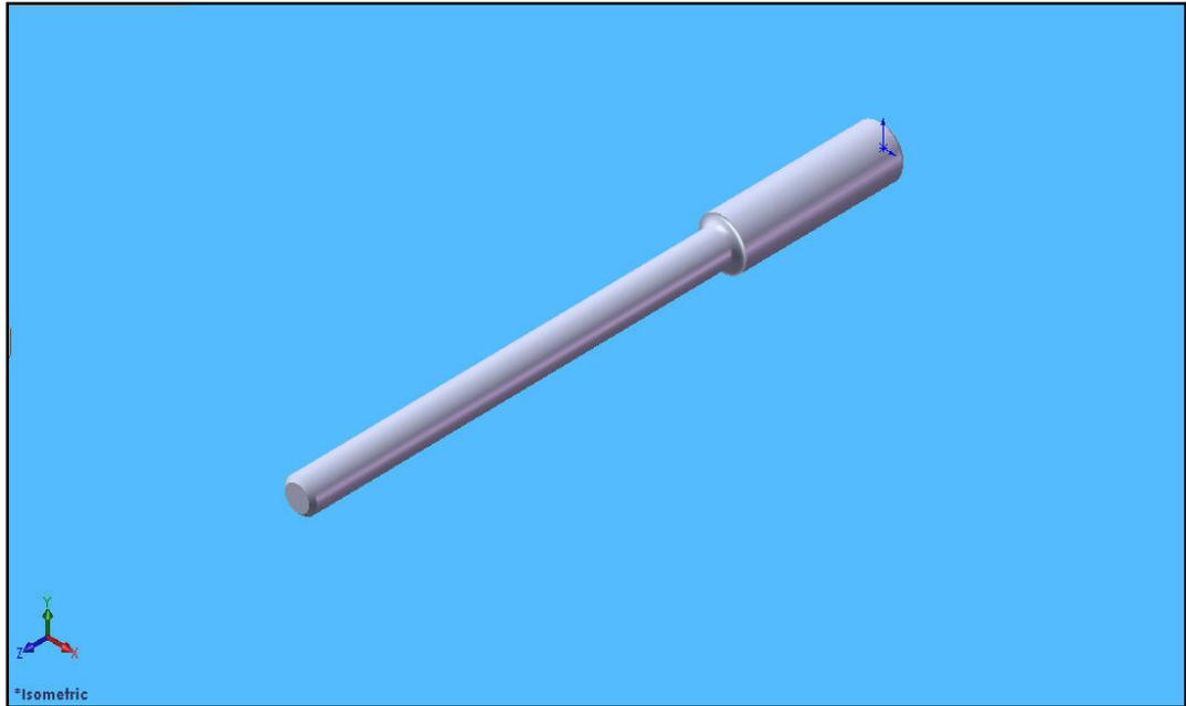
**Figure 3.2:** Fatigue test specimen
