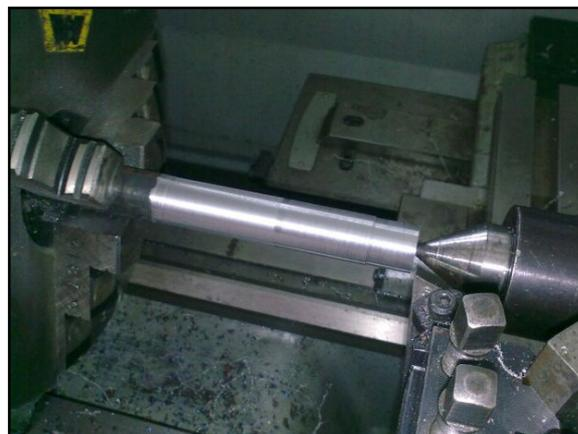
**Figure 3.5:** Turning process
