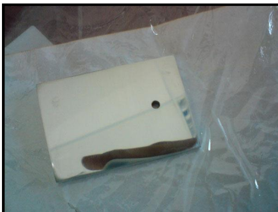
Figure 3.19: Specimen for immersion Test
