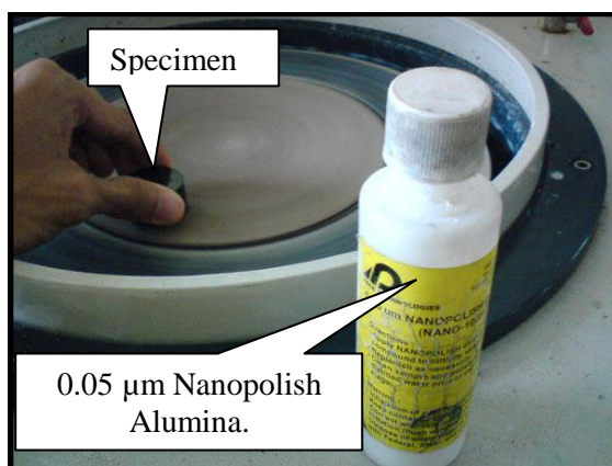
Figure 3.14: Specimens were polish using 0.05 µm NANOPOLISH Alumina.
