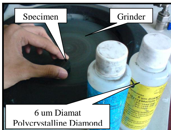
Figure 3.13: Specimens were polish using 6 µm DIAMAT Polycrystalline Diamond followed by 1 µm DIAMAT Polycrystalline Diamond
