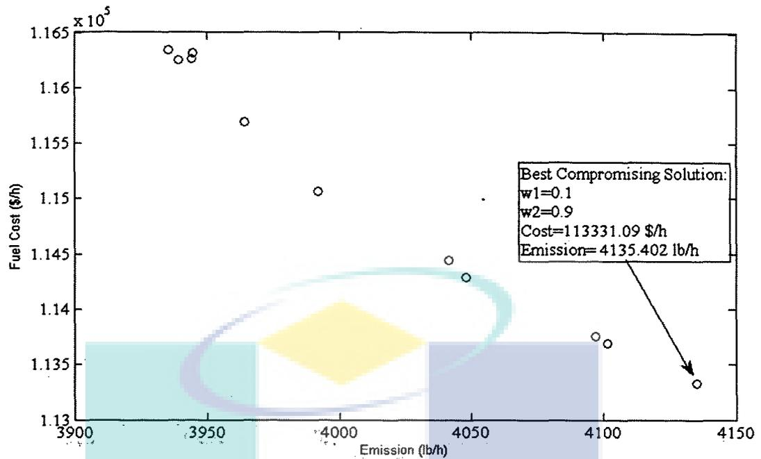
Figure 4.8. Trade-off result using weighted sum method by two decimal value step size for ten generator system with 2000 MW load demand
