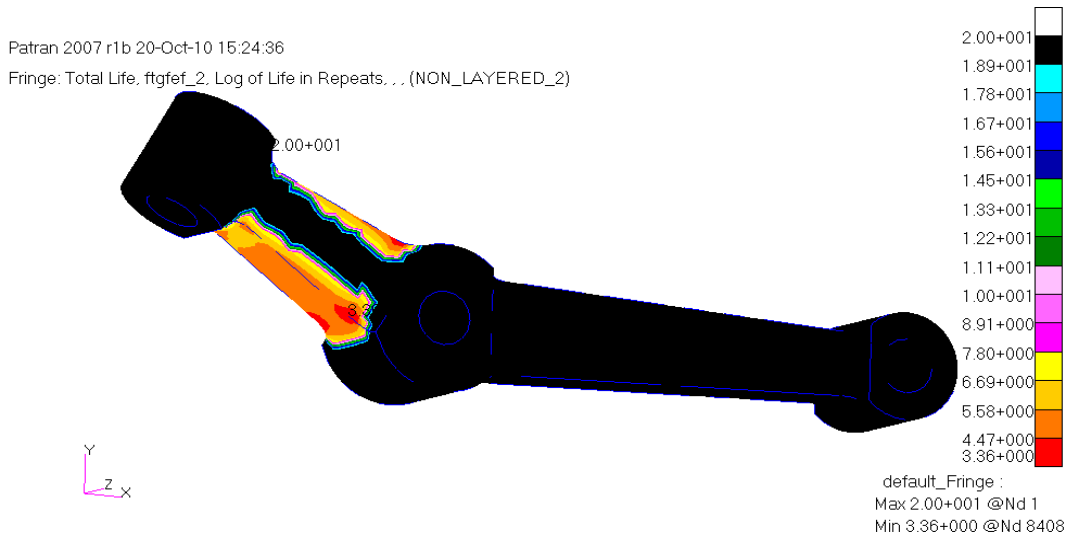
Figure 13: Predicted life contours plotted in term of log of life for 5083-87 aluminum alloy with SAETRN loading by using stress-life method.
