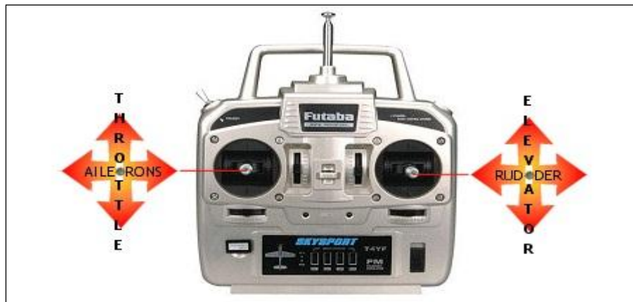
Figure 2.8(c): Radio controller mechanism mode 3
