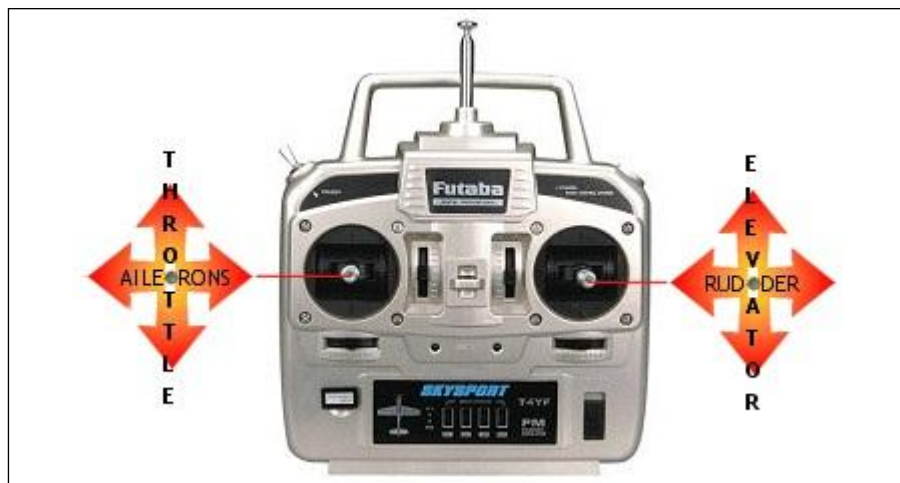
Figure 2.8(d): Radio controller mechanism mode 4
