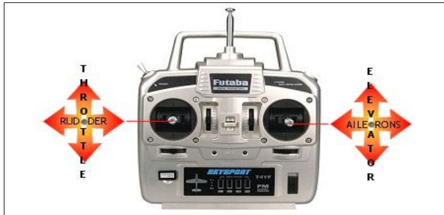
Figure 2.8(b): Radio controller mechanism mode 2
