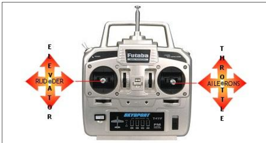
Figure 2.8: Radio controller mechanism mode 1
