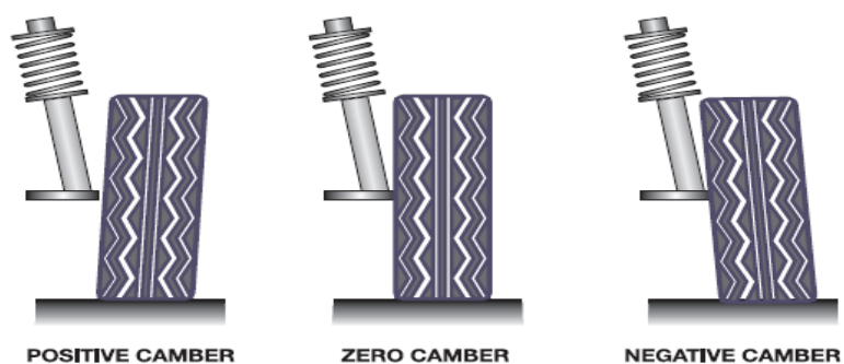
Figure 2.6: Positive, Zero and Negative Camber Angle
