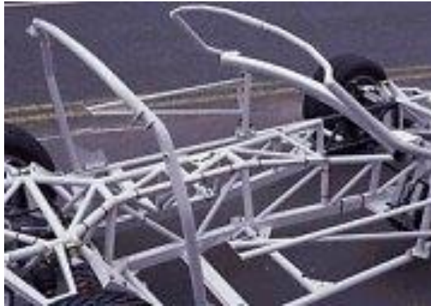
Figure 2.2: An example of chassis of TVR Tuscan
