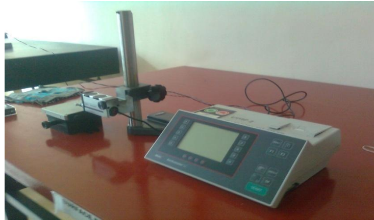
Figure 3.7: Test surface roughness by using Mpi Mhar Perthometer
