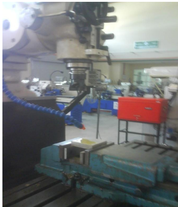
Figure 3.4: Face milling used to rid out rough and wavy surface
