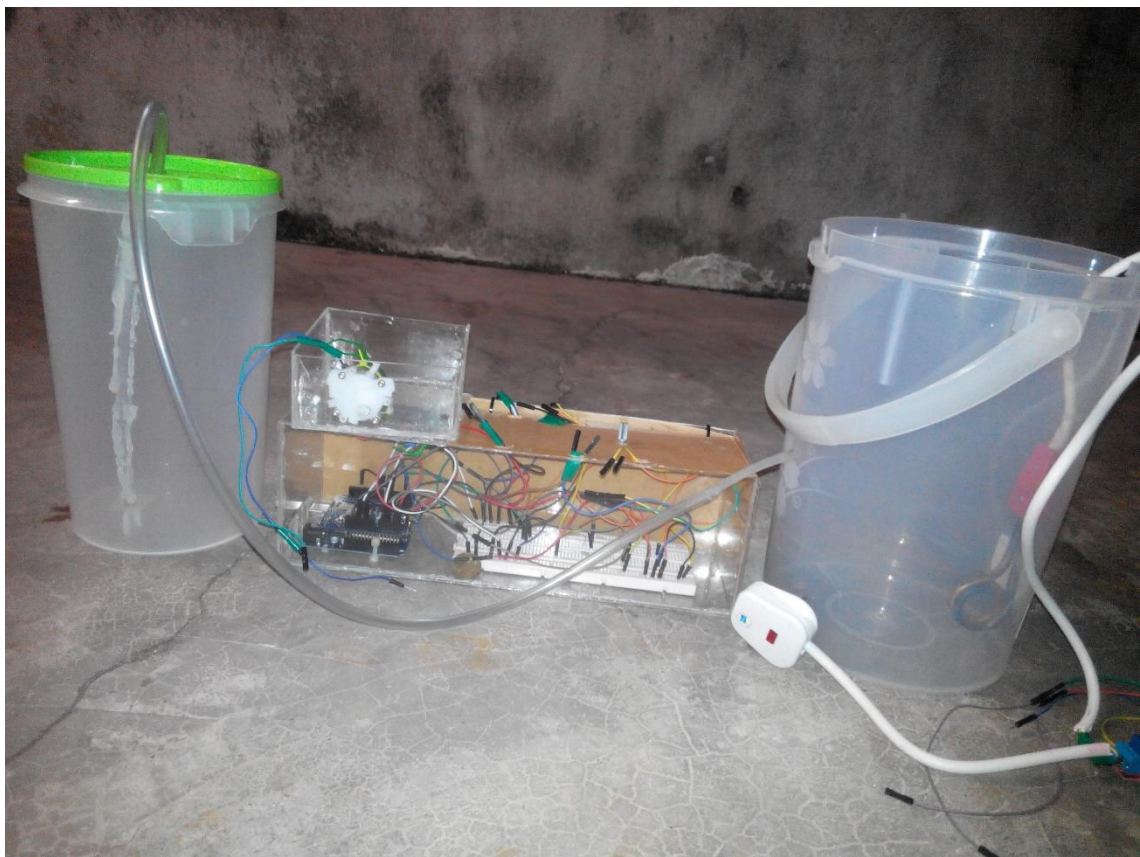
Figure 4.5: The DC water pump hardware setup
