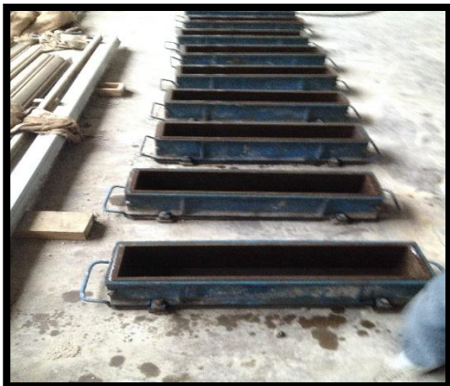
Oil sealed in formwork
