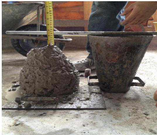
Measured the slump height
