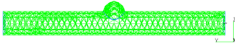
Figure 4.2: The aneurysm design after the meshing process
