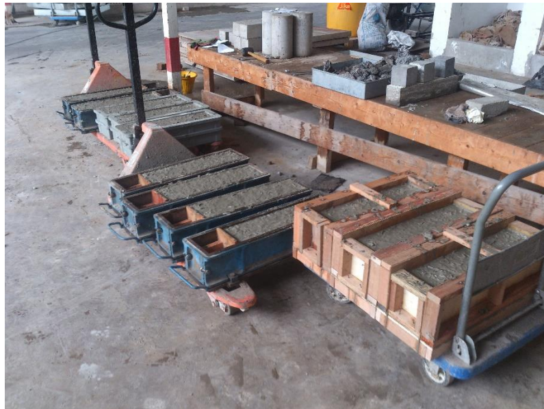
Figure 3.4: Coconut shell concrete in mould
