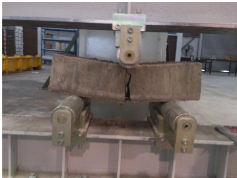
Figure 3.7: Prism after flexural test
