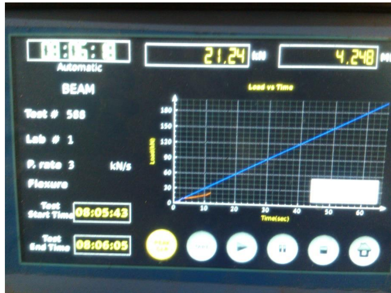
Figure 3.6: Sample reading for NC after flexural test
