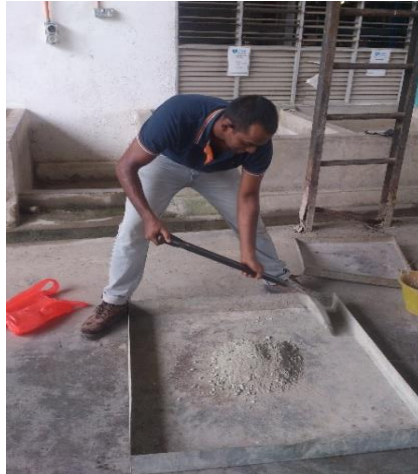
Figure 3.2: Mixing POCC with ratio of 1:1.34:0.89
