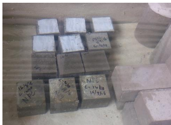
Figure 3.4: Curing process of POCC, immersed in water
