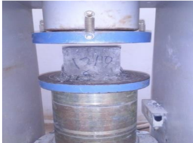
Figure 3.7: Burned POCC carried Compressive strength test
