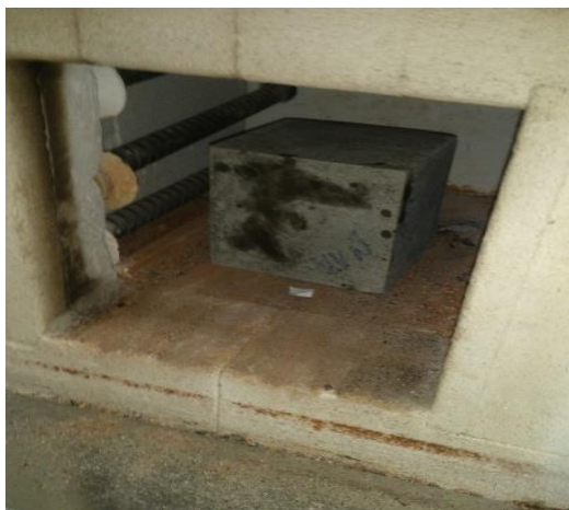
Figure 3.6: Burned POCC at furnace
