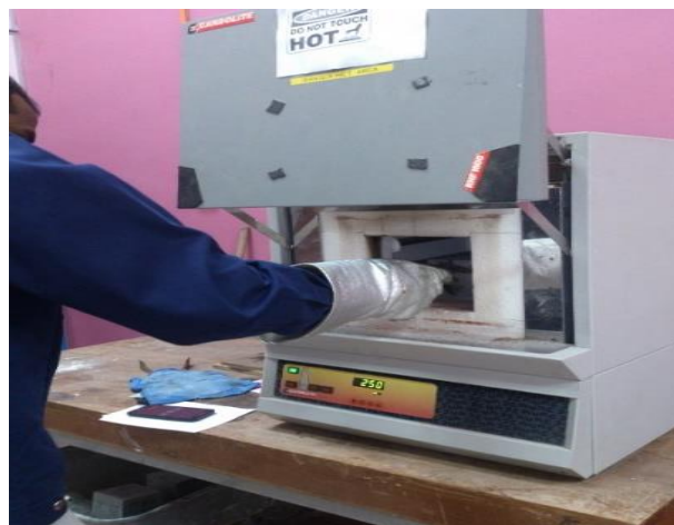
Figure 3.5: POCC sample placed at furnace for burning process.
