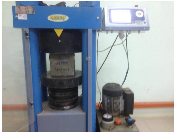
Figure 3.3: Compressive Strength Test
