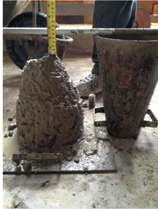
Slump 5% Replacement: 54 mm
