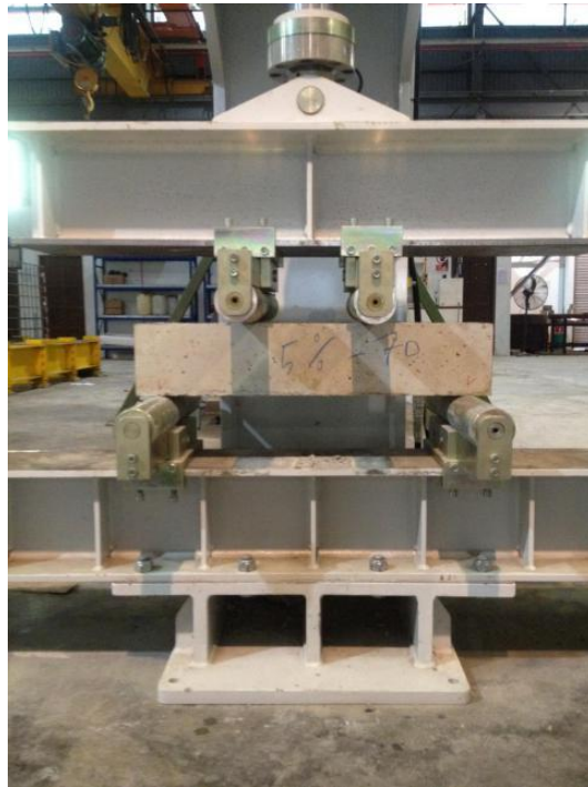
Figure 3.4: Flexural Strength Test
