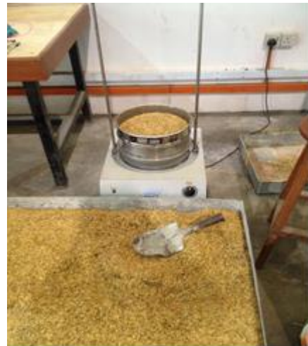
Sieved sample (Passing 4.75 mm)
