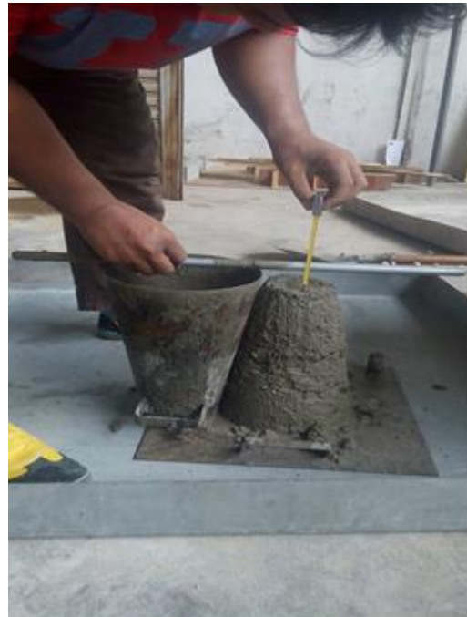
Slump 15% Replacement: 43 mm
