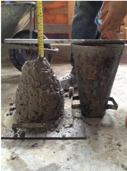
Slump 10% Replacement: 53 mm
