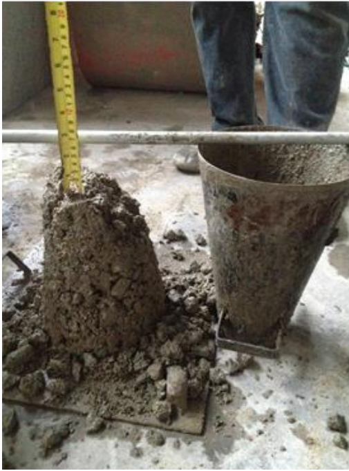
Slump Control: 64 mm
