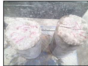
(b) The crack pattern cylinder samples of 2.5% for 7 days
