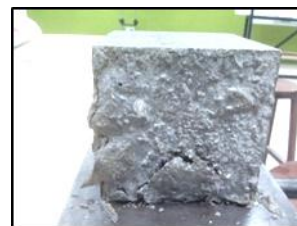
(c) The crack patters cube sample of 5.0% for 14 days
