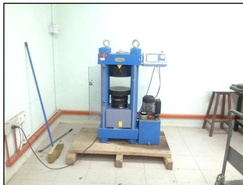
Figure 2.7: Compressive strength machine
