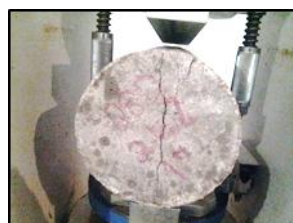
(b) The crack pattern cylinder sample of 2.5% for 28 days
