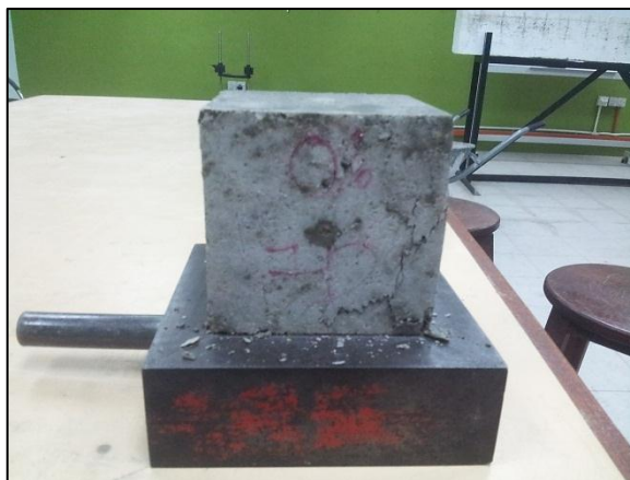
Figure 3.23: The cracking pattern front side of the cube
