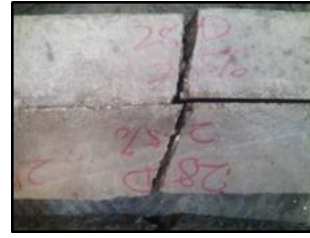
(b) The crack pattern beam samples of 2.5% for 28 days
