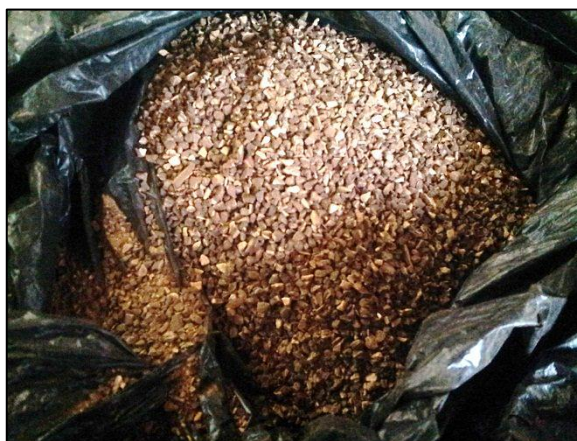
Figure 3.4: Coconut shells were crushing using grinder machine
