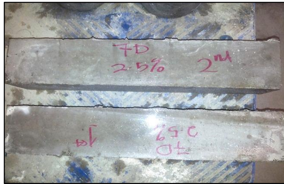
Figure 3.27: Sample of beams was used for flexural strength test based on curing day
