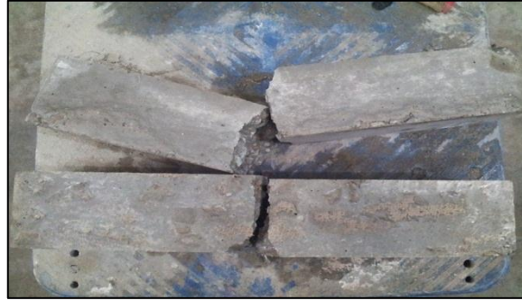
Figure 3.29: The beams specimens after the flexural strength test
