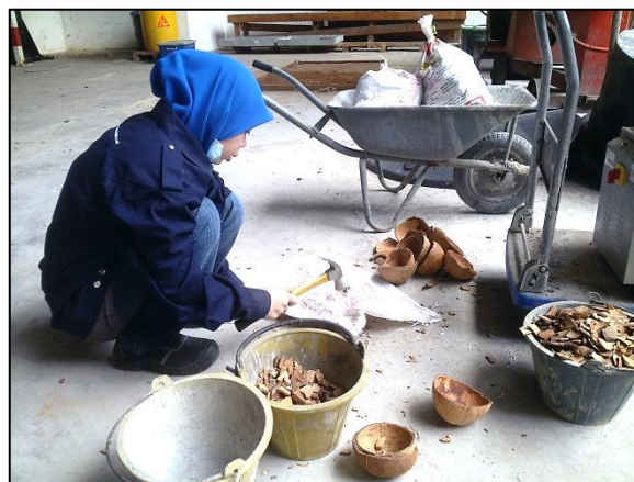
Figure 3.2: Process of crushing coconut shell using hammer
