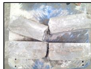
(b) The crack pattern beam samples of 2.5% for 7 days
