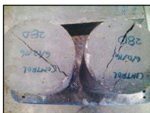
(a) The crack pattern cylinder samples of 0% for 28 days
