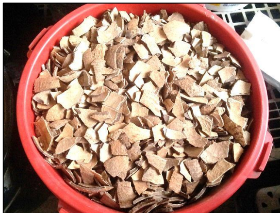
Figure 3.3: Coconut shells were crushing using hammer
