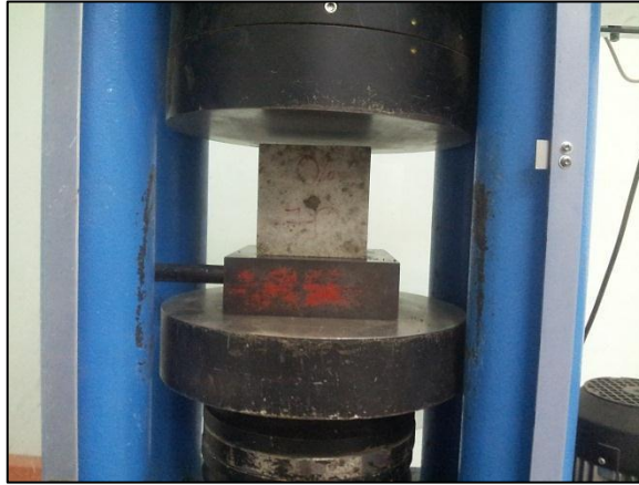
Figure 3.22: The process of compression test
