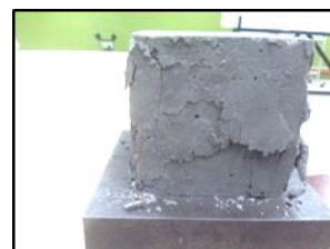
(c) The crack patters cube sample of 5.0% for 28 days
