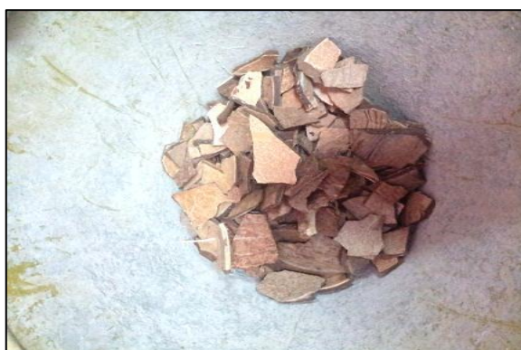
Figure 2.5: Coconut shell as replacement of coarse aggregate
