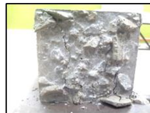
(e) The crack patters cube sample of 10% for 14 days
