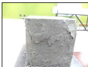
(b) The crack patterns cube sample of 2.5% for 2 days
