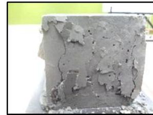
(e) The crack patterns cube sample of 10% for 7 days
