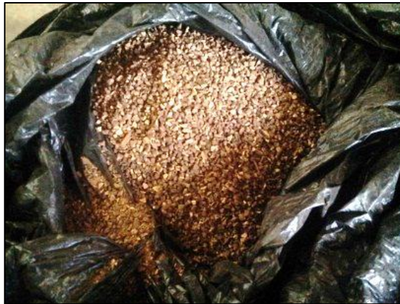
Figure 2.6: Coconut shell as replacement of fine aggregate
