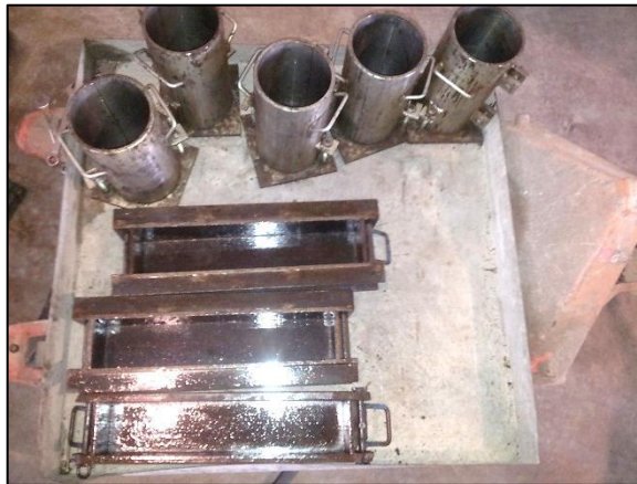
Figure 3.9: Preparation of beam and cylinder moulds for splitting tensile and flexural strength test
