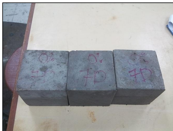
Figure 3.21: Sample of the cubes was used for compression test based on curing day.
