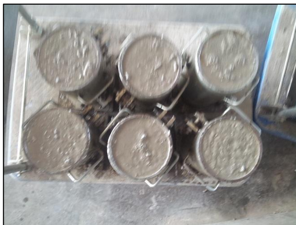
Figure 3.18: Casting concrete for cylinders already done
