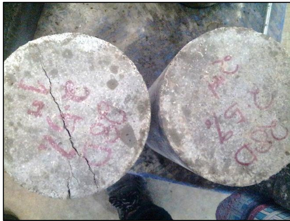
Figure 3.26: The cracking pattern of cylinders after splitting tensile test
