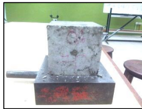
(a) The crack patterns of cube sample of 0% for 7 days
