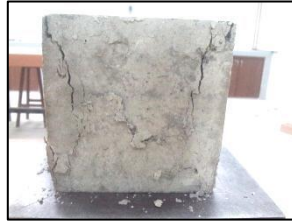
(a) The crack pattern of cube sample of 0% for 14 days
