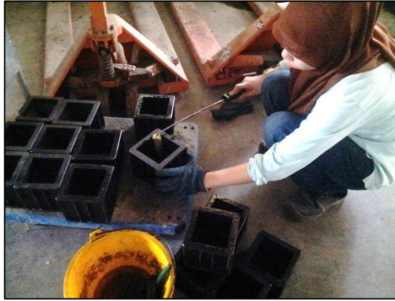
Figure 3.8: Preparation on cube moulds for compressive test
