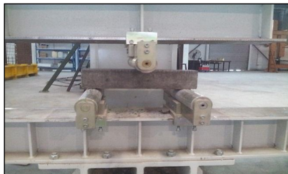
Figure 3.28: The process of flexural strength testing
