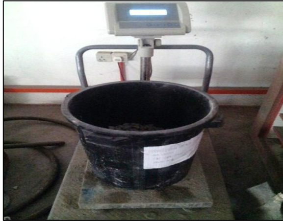
Figure 3.10: Weighing all the materials that used in concreting process
