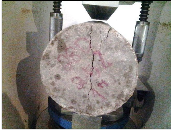
Figure 3.25: The process of splitting tensile test
