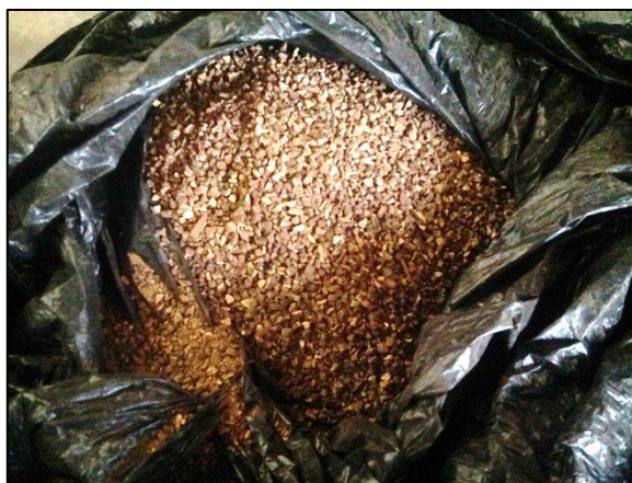
Figure 3.6: Size of coconut shells passing the 5 mm sieve as a replacement on fine aggregate
