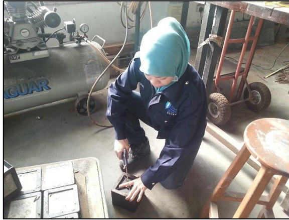
Figure 3.19: The process of remoulding concretes
