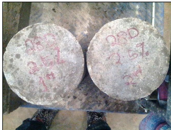
Figure 3.24: The cylinders are conducted on the splitting tensile test based on curing day
