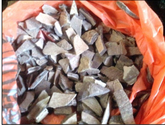
Figure 3.7: Size of coconut shells passing 10 mm and 20 mm sieve as a replacement of coarse aggregate
