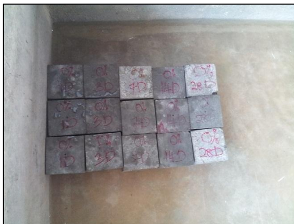
Figure 3.20: The curing process of cubes, beams and cylinders after remolding
