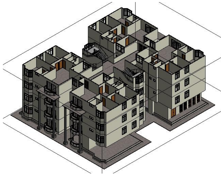
Plan view cross section by using section box
