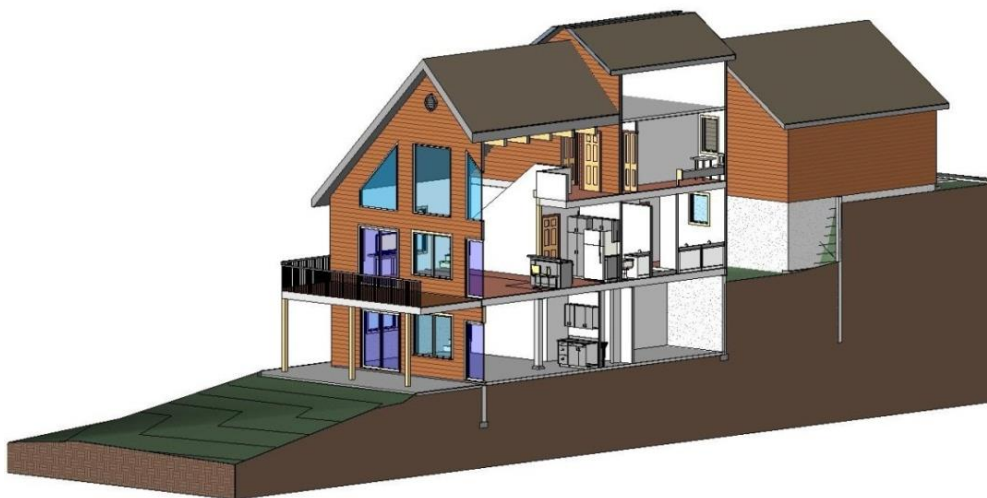
Figure 2.5: 3D cross sections produced by BIM (Monahan Design LLC, 2016)
