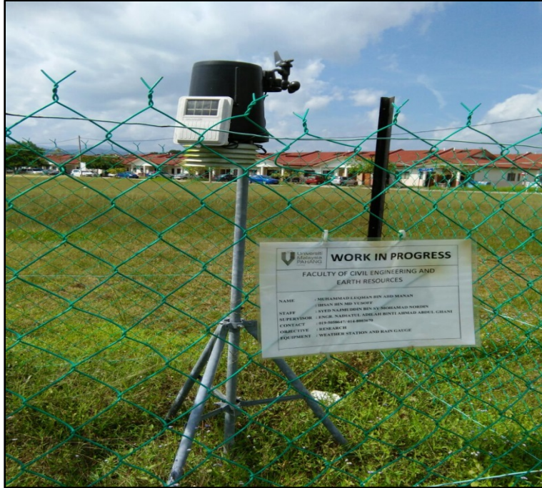
Figure 3.9: Wireless Vantage Pro ISS with Fan-Aspirated Shield
