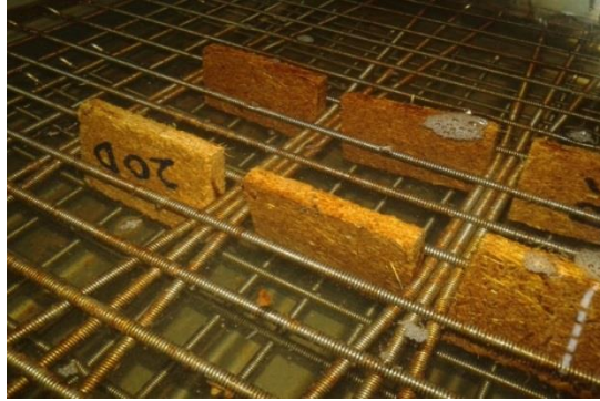
Figure 3.10 Water absorption and thickness swelling test
