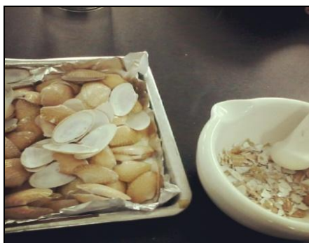
Figure 3.2. Paphia Undulata shell chruishing process.
