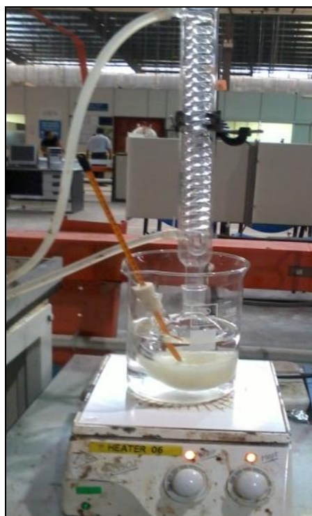
Figure 3.4. Esterification of Jatropha curcas oil.
