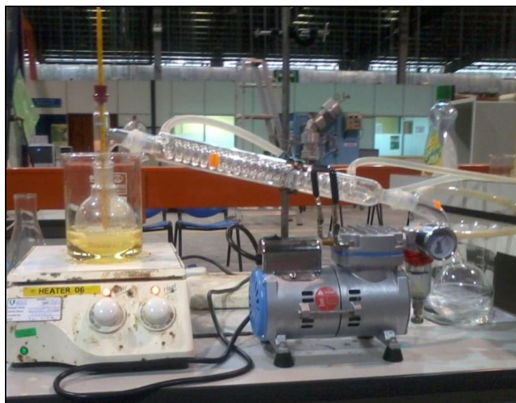
Figure 3.8. Experimental setup for biolubricant synthesis.
