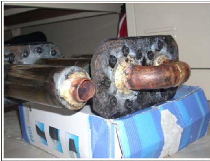
Figure 4.14: Rear end head welding
