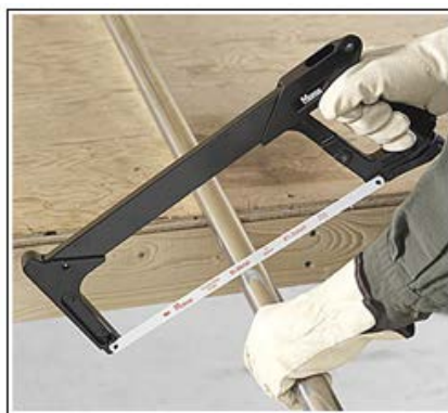
Figure 4.7: Sawing on stainless steel pipe
