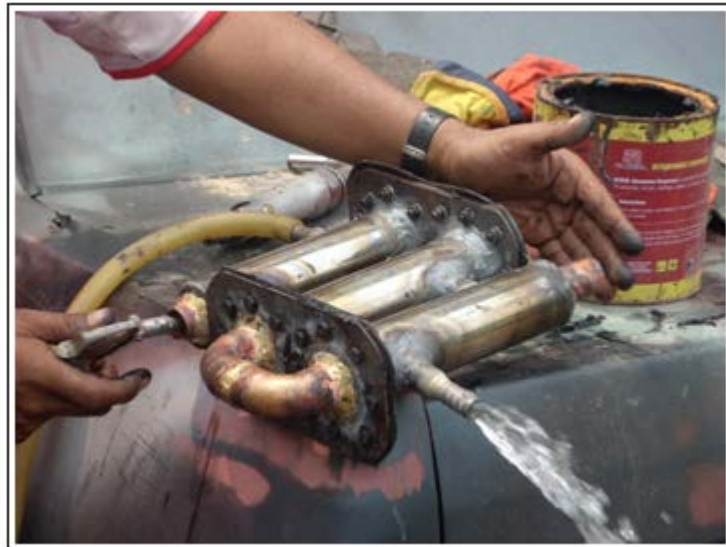
Figure 4.16: Heat exchanger air/water test
