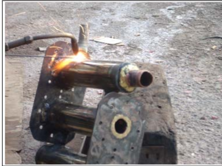
Figure 4.10: Welding on stainless steel pipe and small steel pipe
