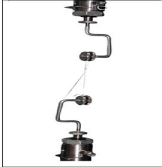
Figure 3.2: O-Ring Fiber Clamping Grip
