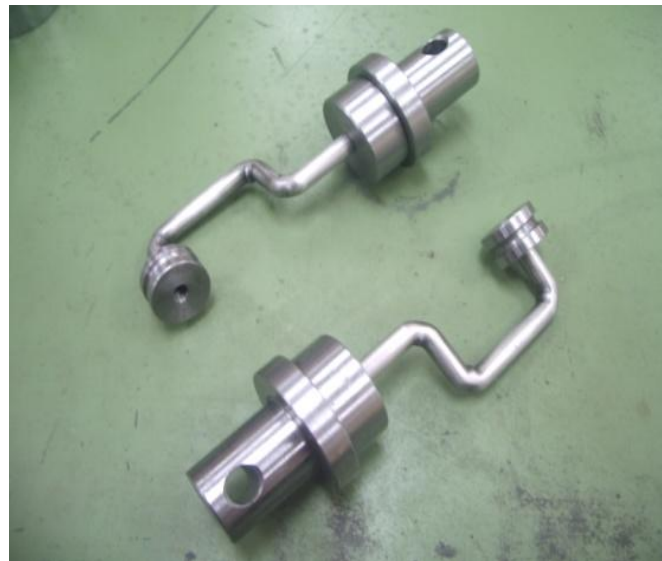
Figure 3.5: O-Ring fiber clamping grips
