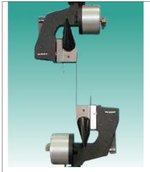
Figure 2.5: Pneumatic cord and yarn style grips
