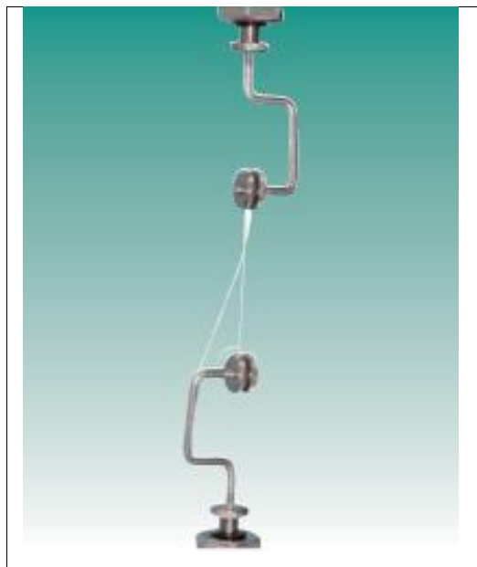
Figure 2.4: O-Ring fiber clamping grips
