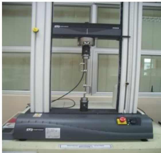
Figure 6.10: Assembling of tensile test rig and universal testing machine
