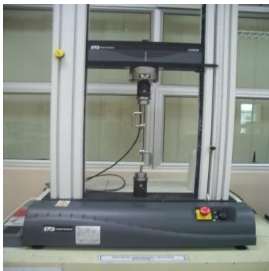
Figure 3.7: Alignment of the clamps
