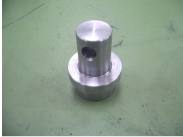
Figure 6.5: Clevis Interface Part
