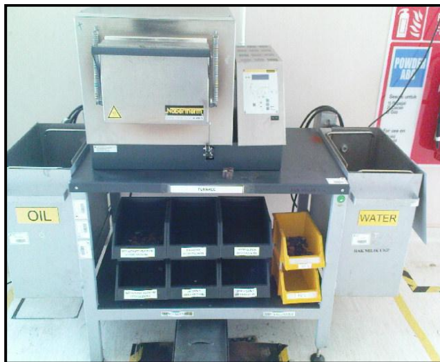
Figure 3.3: Furnace for stress relieving process
