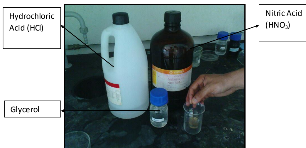
Figure 3.7: Etching solution 20 ml hydrochloric acid (HCl), 20 ml glycerol and 10 ml nitric acid (HNO 3 )
