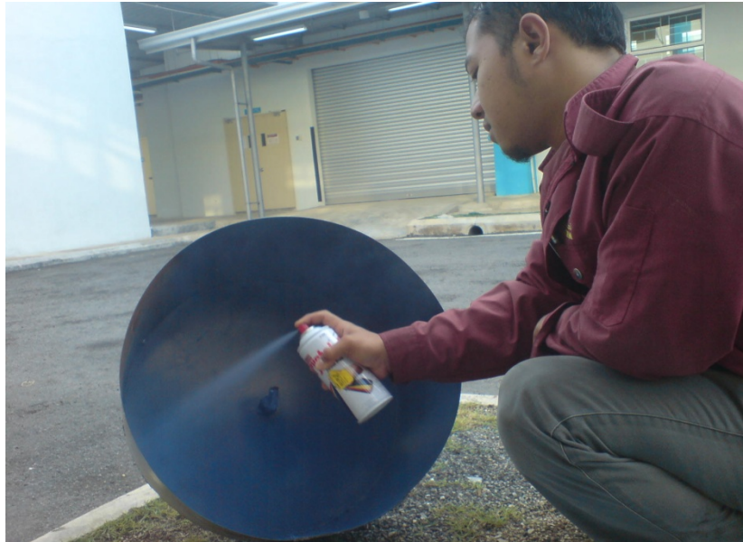
Figure 3.10: Spraying process with anti-rust
