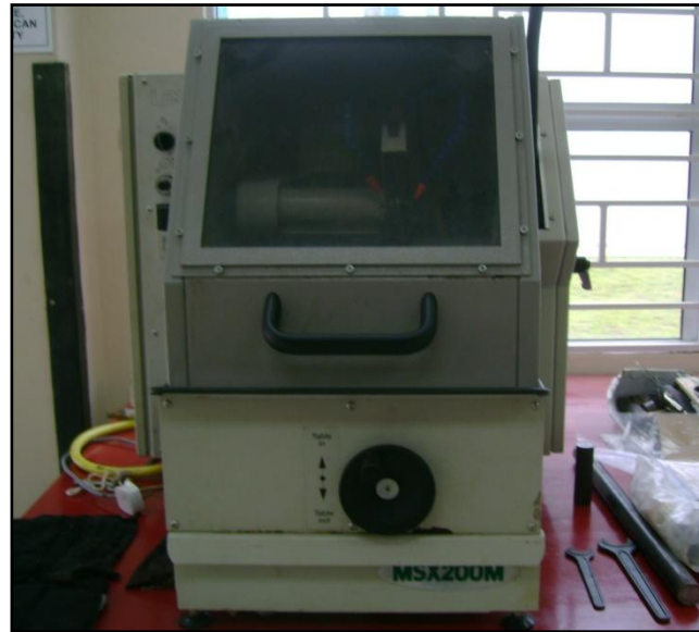
Figure 3.3: Sectioning cut-off machine
