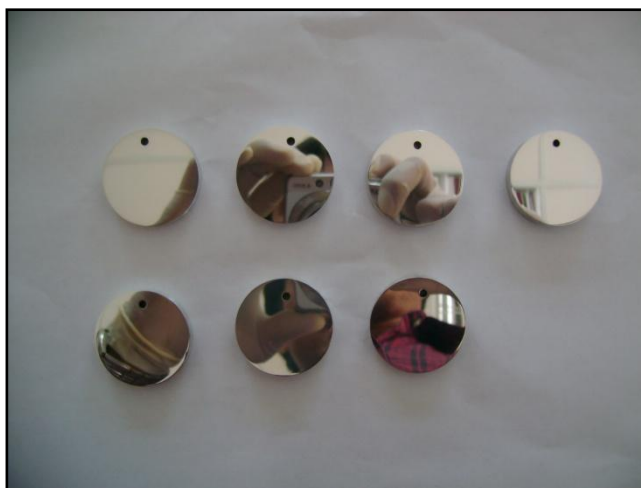
Figure 3.6: The samples after polishing process
