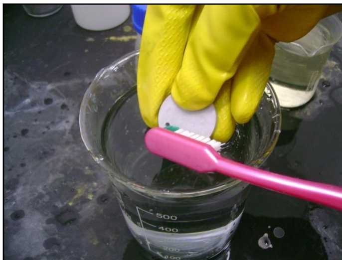
Figure 3.12: Cleaning process via Nitric acid by light brushing
