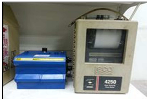
Figure 3: ISCO 2150 and 4250 Area Velocity Flowmeter
