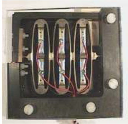
Figure 2.5: MRI compliant 3mm-stroke mechanism based on three APA200M-NM's. The actuator is actuated at 180V DC and displaying its maximum stroke.
