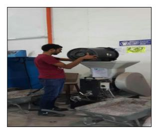
Figure 2: Palm oil clinker pulverizing process
