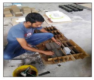
Figure 5: Casting of brick specimen
