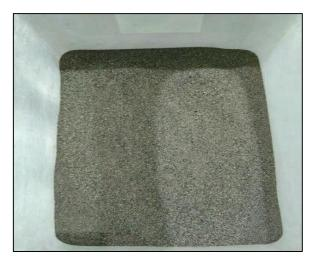
Figure 4: Fine palm oil clinker after grinding
