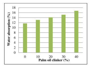
Figure 10: Water absorption result at 28days
