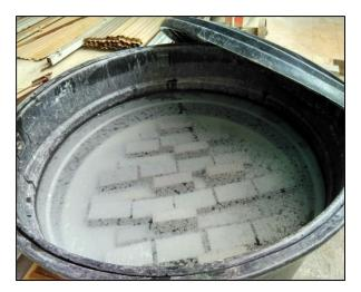
Figure 6: Specimen subjected to water curing
