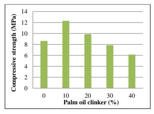
Figure 8: Compressive strength result up to 28days
