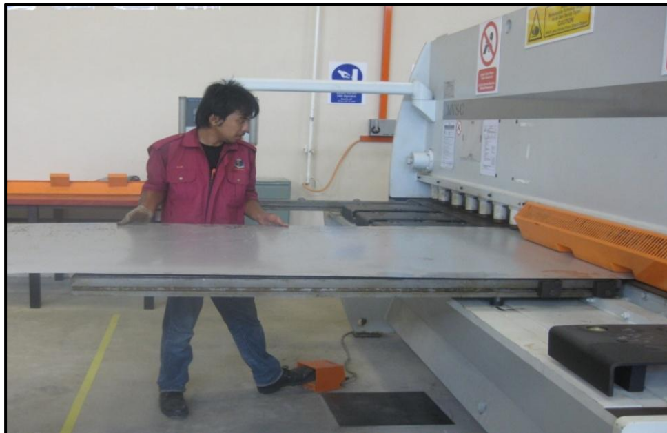
Figure 3.3: Cutting process with shearing machine
