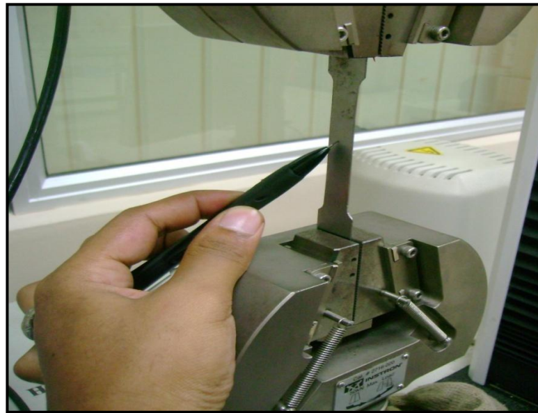
Figure 3.9: Sensor calibration by using pencil break test
