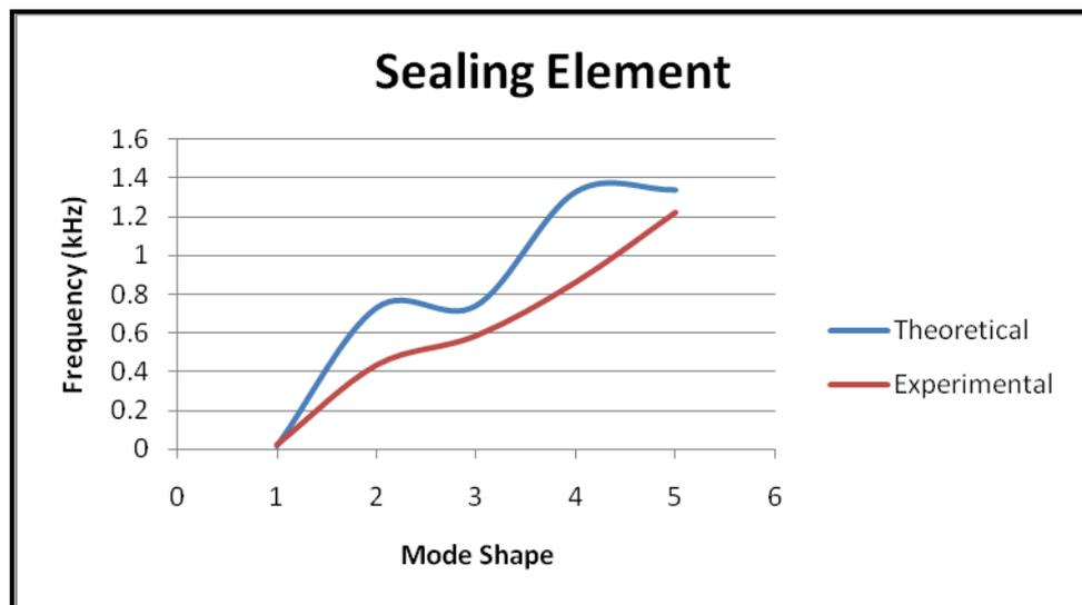
**Figure 4.8:** Comparison result for sealing element**Table 4.9:** Natural frequencies analysis of inner ring
