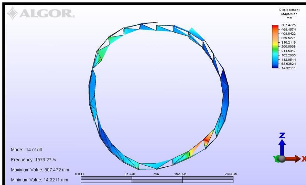
Figure 6.18: Mode shape 4 of inner ring
