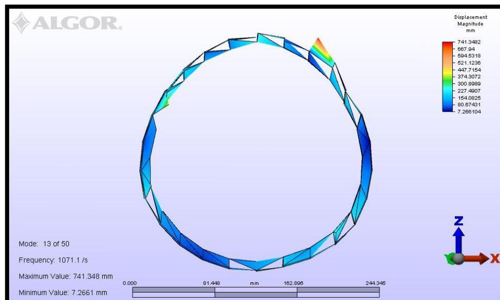
**Figure 6.17:** Mode shape 3 of inner ring
