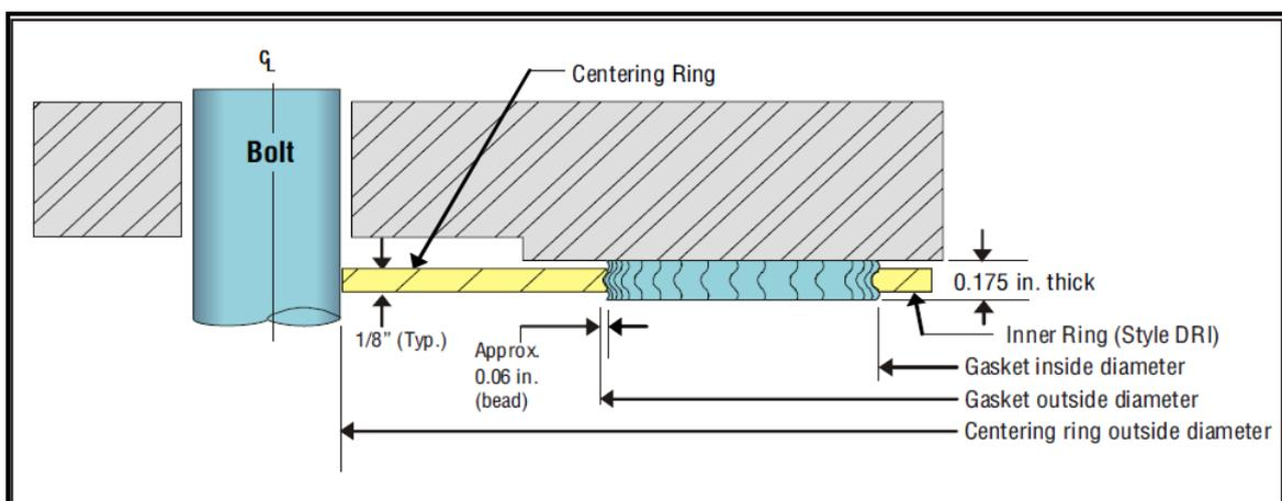
**Figure 2.4:** Spiral wound gasket installation
