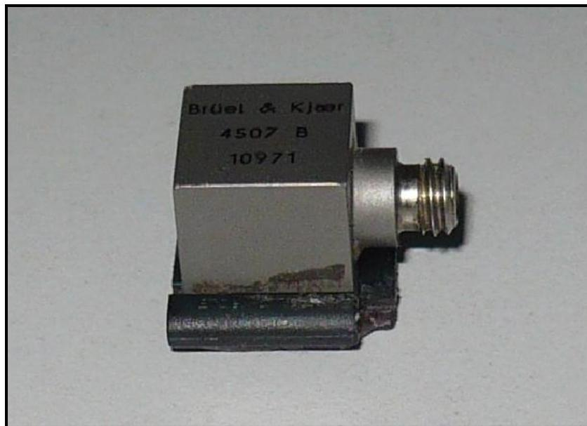
**Figure 3.16:** Accelerometer
