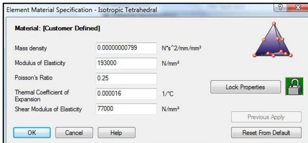
**Figure 3.8:** Material Specification
