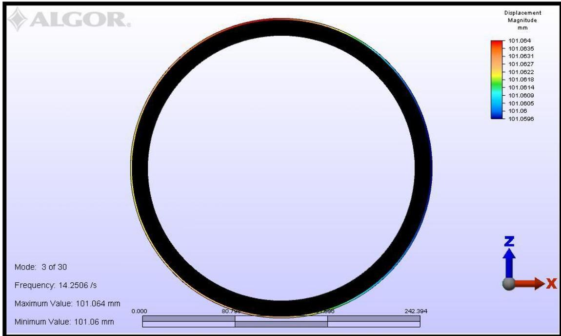
**Figure 4.2:** Sealing element mode shape
