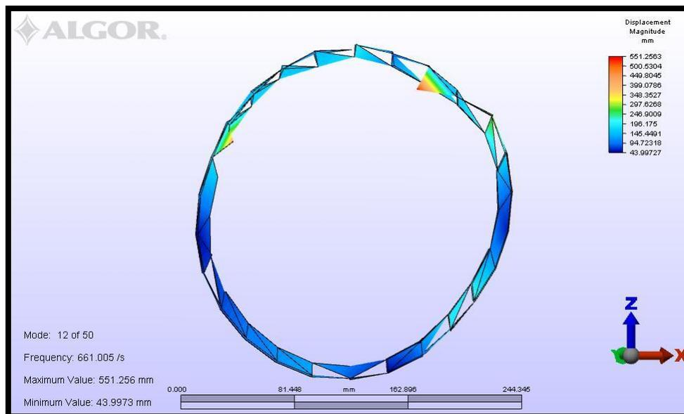
**Figure 6.16:** Mode shape 2 of inner ring
