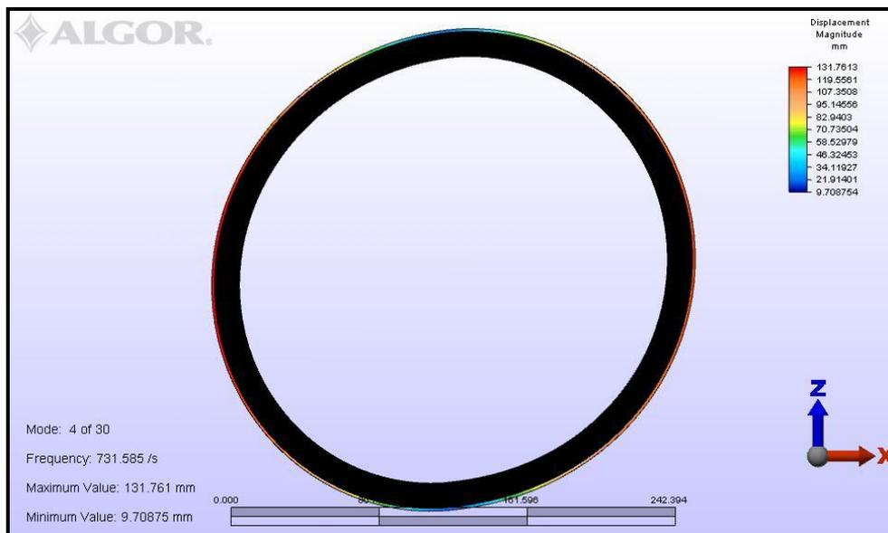
**Figure 6.12:** Mode shape 2 of sealing element
