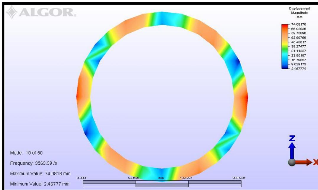
**Figure 6.10:** Mode shape 4 of outer ring
