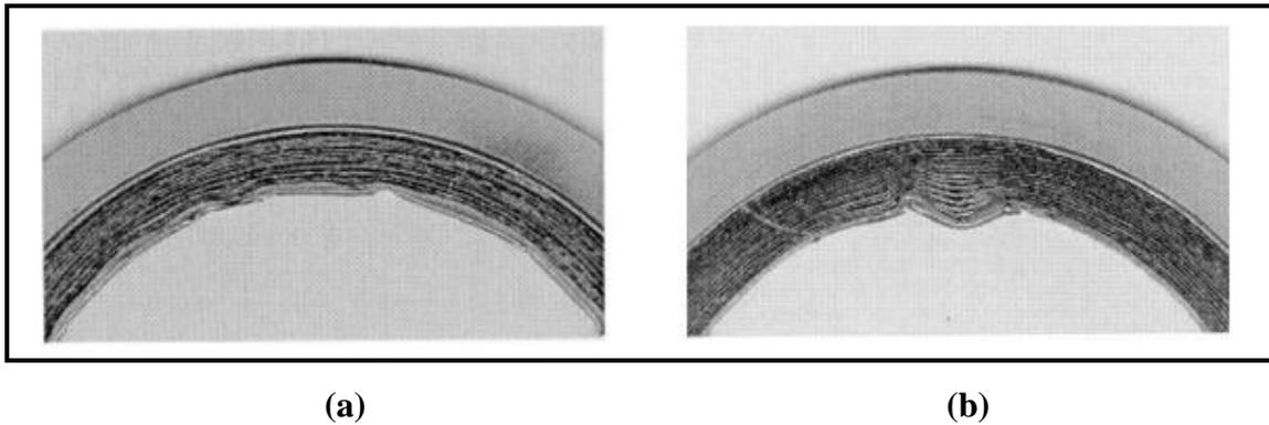
**Figure 2.6:** (a) Uniform radial buckling. (b) Localized buckling.
