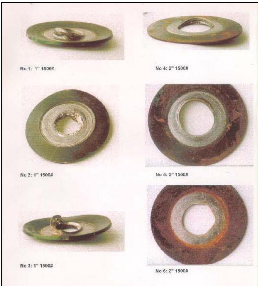
**Figure 6.1:** Spiral wound gasket failure
