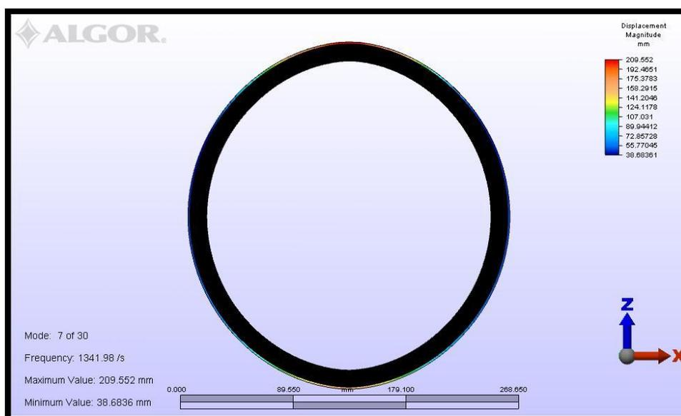
**Figure 6.15:** Mode shape 5 of sealing element
