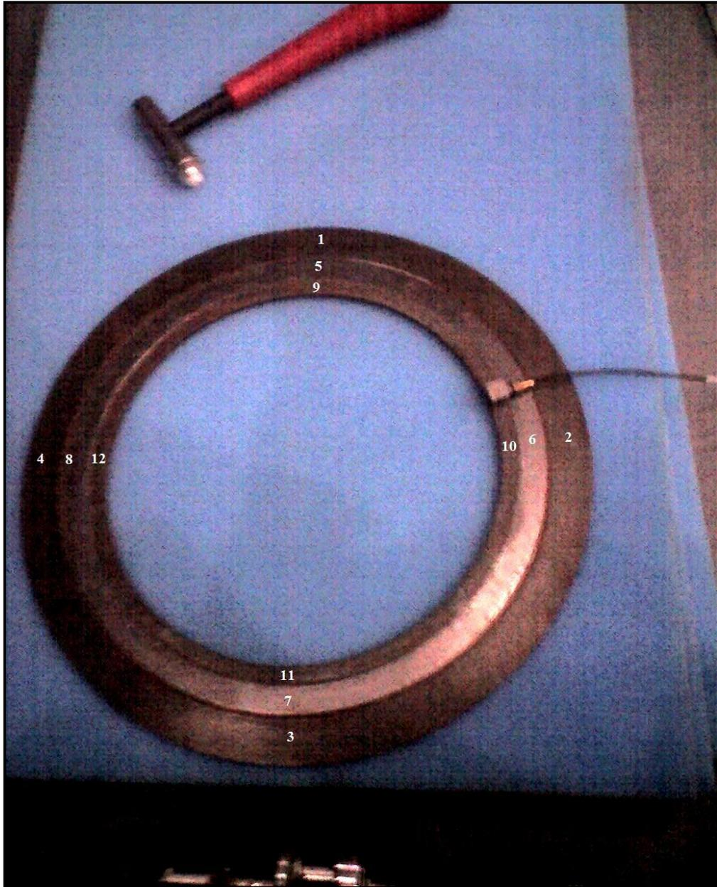
**Figure 3.20:** Impact hammer testing on a spiral wound gasket
