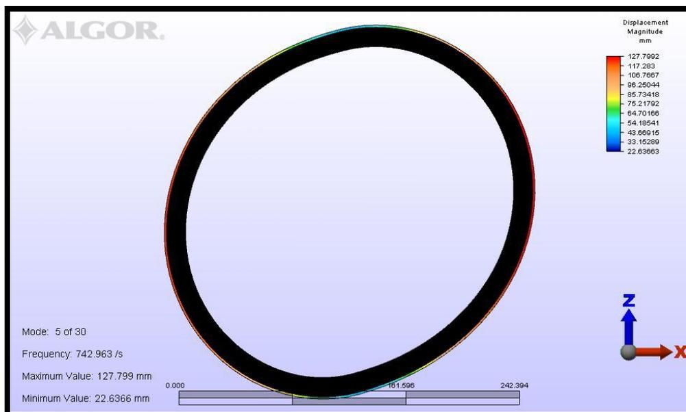
**Figure 6.13:** Mode shape 3 of sealing element
