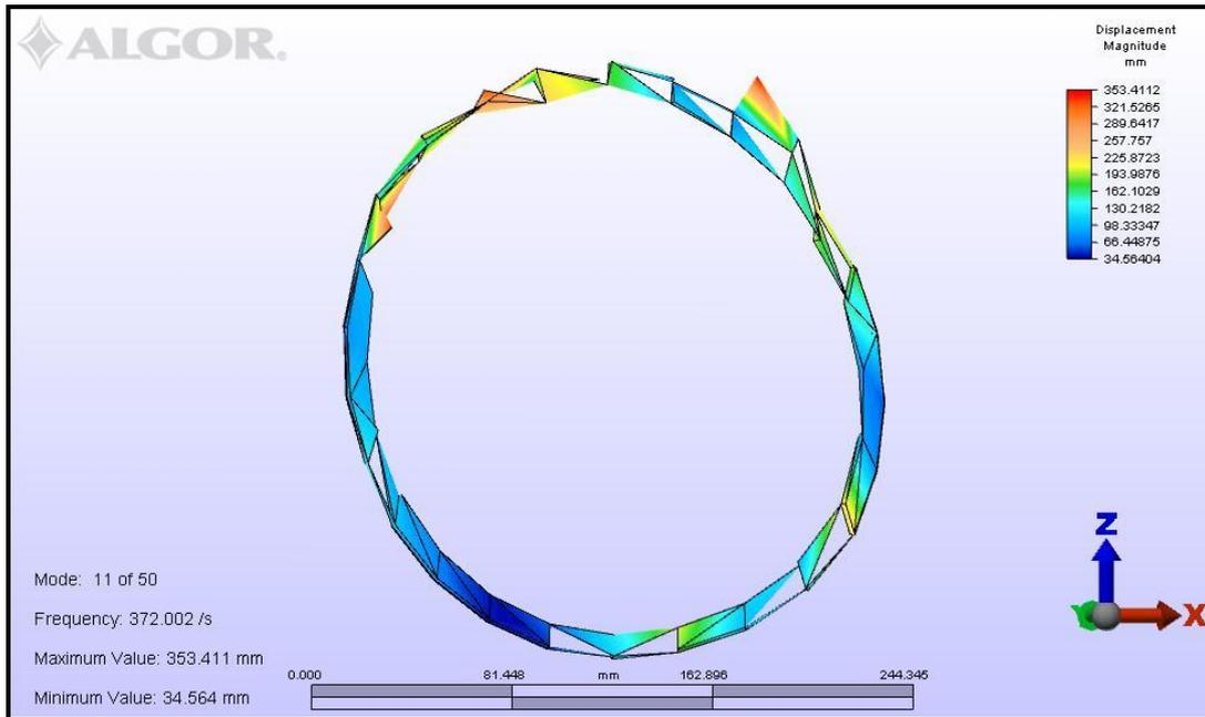
**Figure 4.3:** Inner ring mode shape
