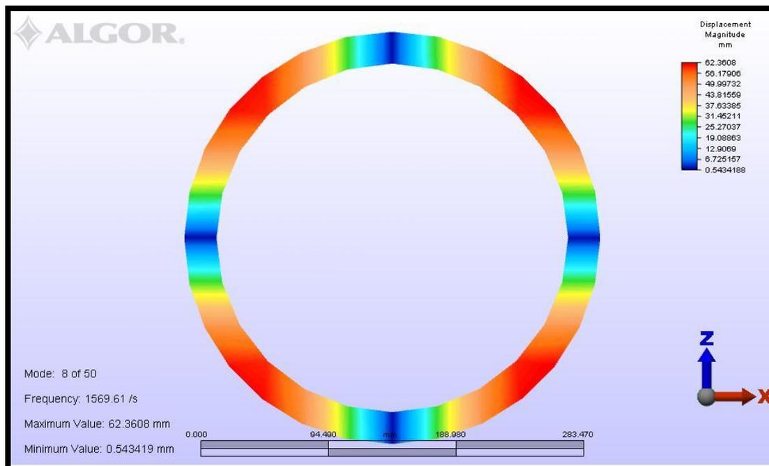
**Figure 6.8:** Mode shape 2 of outer ring
