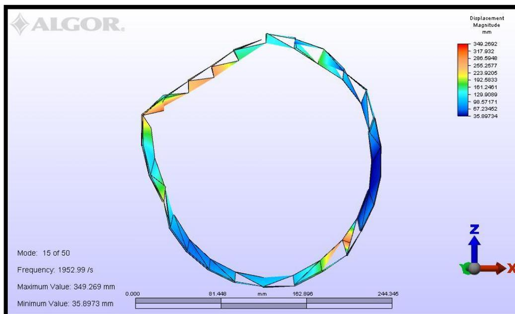
Figure 6.19: Mode shape 5 of inner ring
