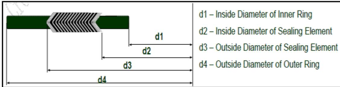
**Figure 3.3:** Diameter of the spiral wound gasket
