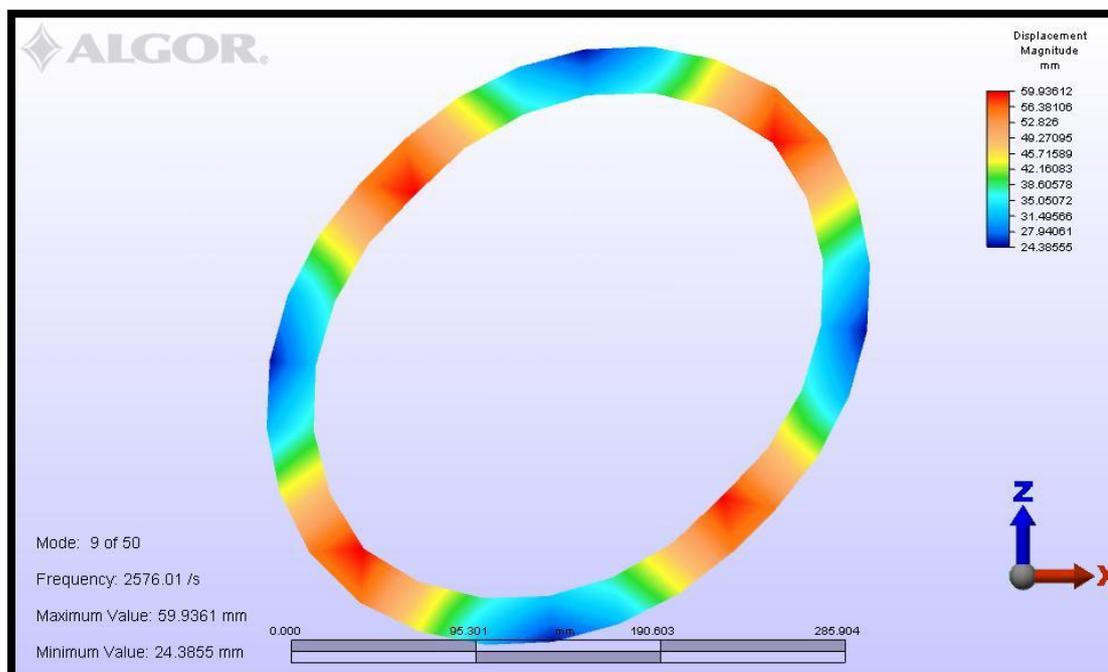
**Figure 6.9:** Mode shape 3 of outer ring
