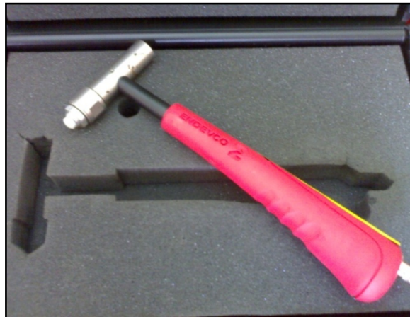
Figure 3.11: Modal hammer Model: 2302-10, Endevco
