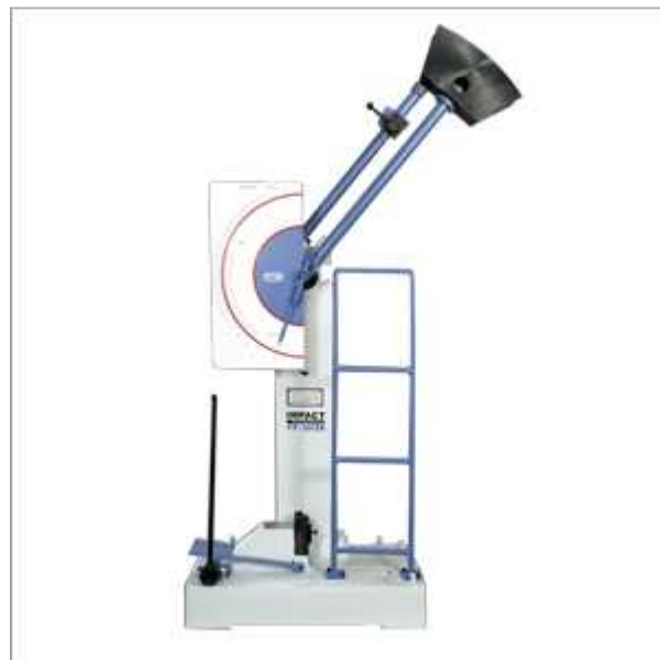
Figure 2.4: Analog Charpy Izod Impact Testing Machine FIT 300
