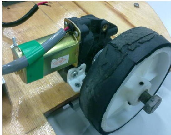
Figure 3.3: Attachment between tires and power windows motor.
