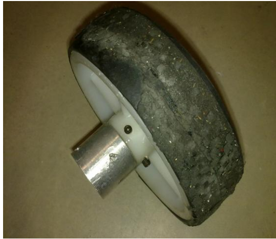
Figure 3.2: Attachment between shaft and tire.
