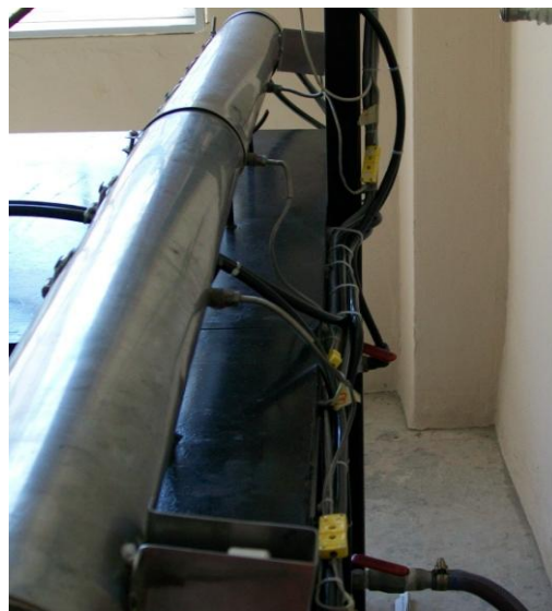
(b) Back view of test section with heaters and thermocouples
