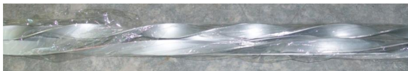
Figure 3.13 : Twisted tape insert
