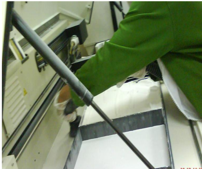
Figure 3.8: Clean the service station
