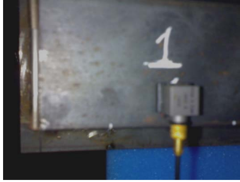
Figure 3.9 : Excitation measurement on the first point using accelerometer
