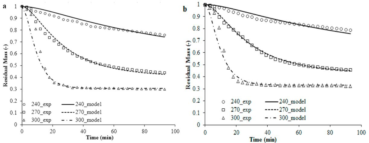
Fig. 2. AWL modelling for (a) Cengal ; (b) Kulim wood sawdust at all temperature with heating rate 10°C/min during torrefaction
