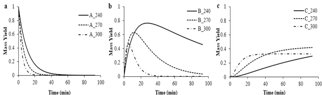
Fig. 4. Mass yield of (a) A (Biomass); (b) B (Intermediate); (c) C (Char) for Kulim wood sawdust at all temperature
