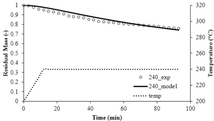
Fig. 1. Experimental and modeled result of Cengal sawdust torrefaction at 10°C/min heating rate
