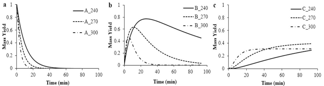
Fig. 3. Mass yield of (a) A (Biomass); (b) B (Intermediate); (c) C (Char) for Cengal wood sawdust at all temperature
