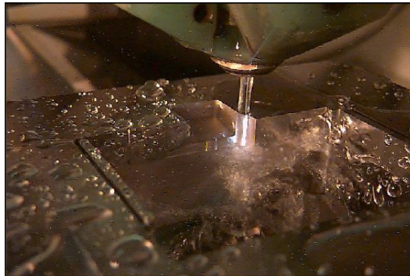
Figure 2.4: An example of wire EDM
