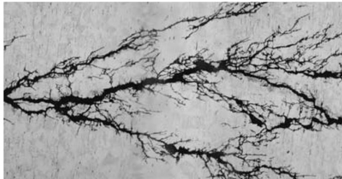
Figure 2.7: Corrosion due to crack that formed by tensile stress [1]
