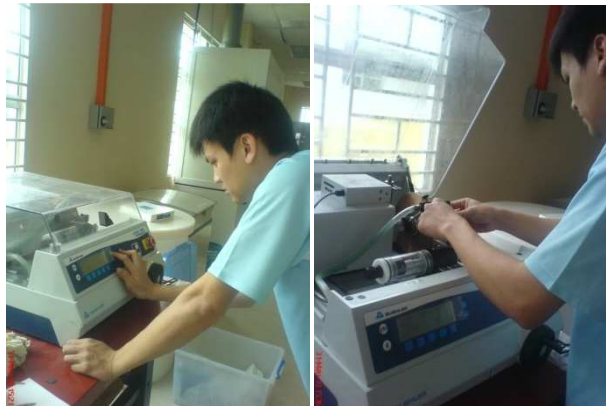
Figure 3.6: The operating procedure of Iso Met 4000 Linear Precision Saw machine.
