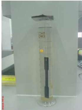
Figure 3.19: The specimen immersed in the cylinder with seawater.
