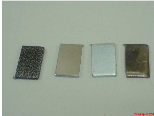
Figure 3.7: The small pieces of the 4 different specimens cut by using Iso Met 4000 Linear Precision Saw machine (From left to right: Powder coating, Nickel electroplating, Zinc electroplating and without coating)
