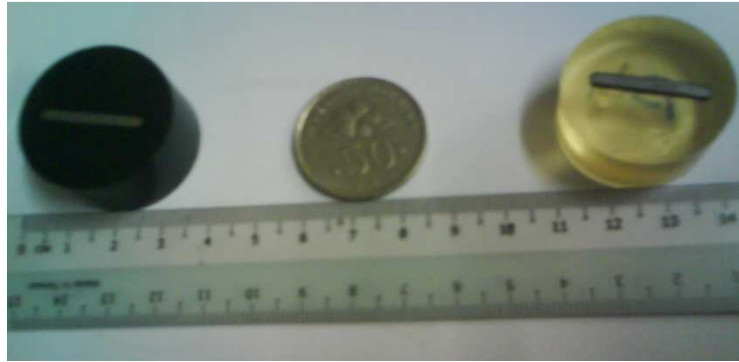
Figure 3.10: The small pieces of the specimen after hot (left) and cold (right) mounting process.
