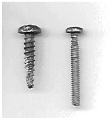
Figure 2.2: Crevice corrosion on the screws. [1]
