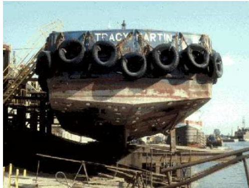
Figure 2.10: Bottom of the boat with cathodic protection to prevent corrosion happen [1]
