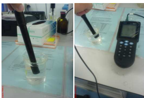
Figure 3.18: The process of taken the reading of salinity.
