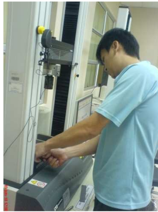
Figure 3.22: The setting up procedure of the INSTRON Universal Testing Machine.
