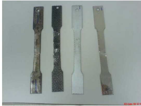
Figure 3.24: The different specimens after the tensile test. (From left to right, without coating, powder coating, zinc electroplating and nickel electroplating)
