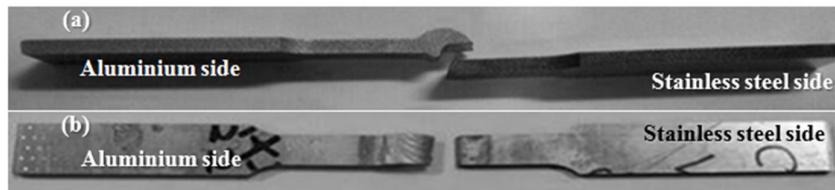
Figure 3. Fractured tensile specimen from the (a) side view, and (b) top view.
