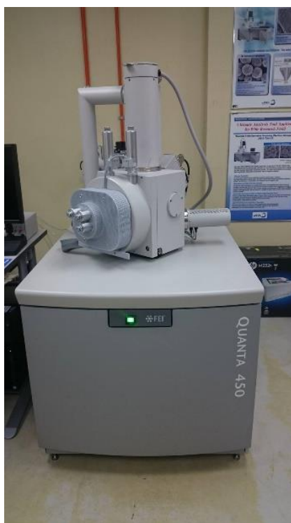
Figure 3.8: Scanning Electron Microscopy, Quanta 450
