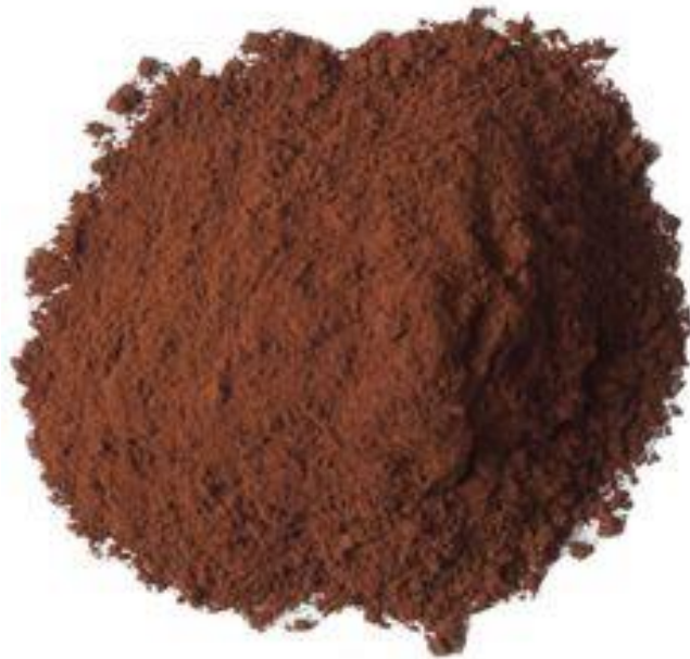
Figure 3.2: Copper zinc ferrite produced after calcined
