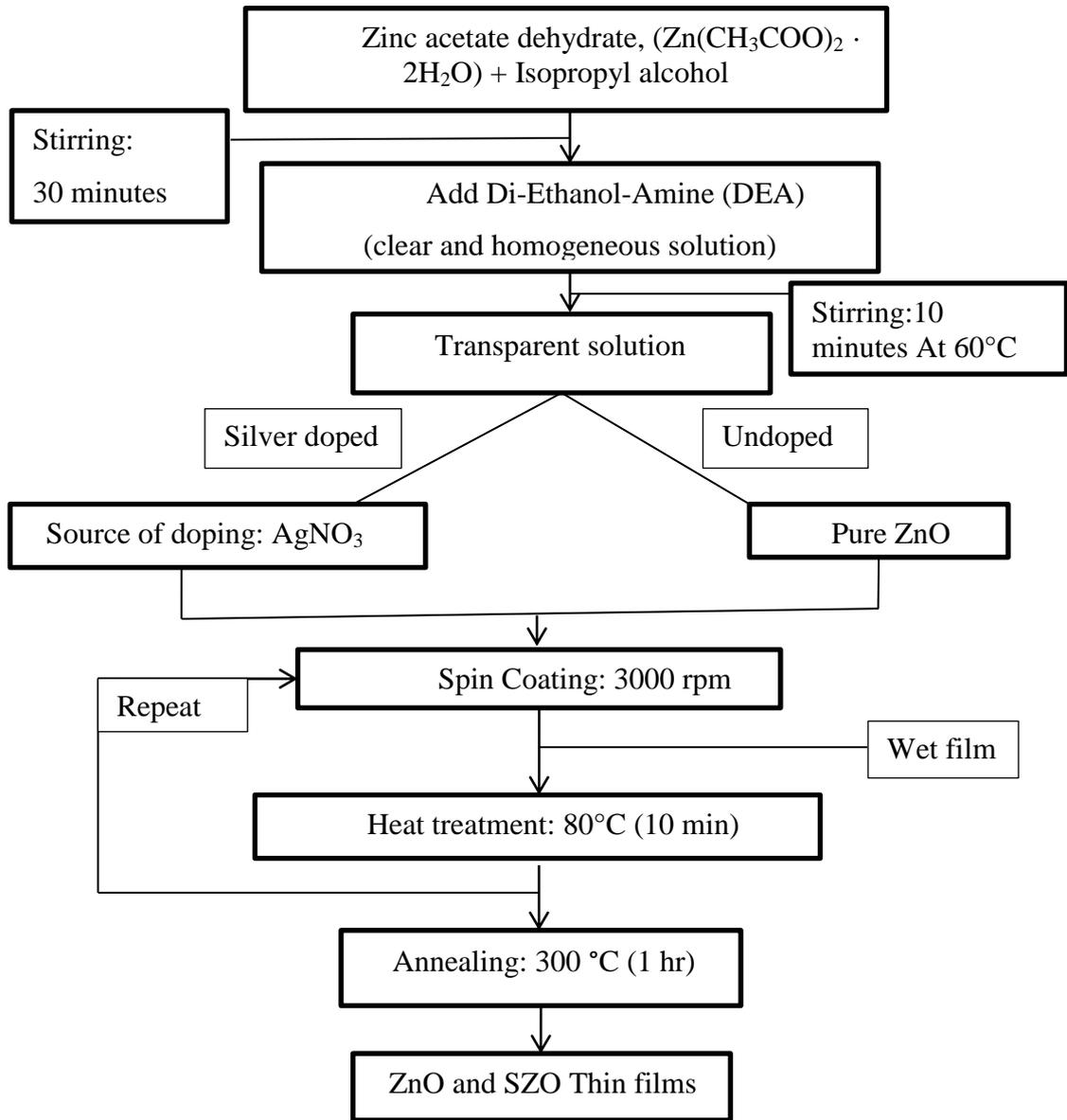
Figure 3.1. Flow chart showing the procedure for preparing ZNO and SZO thin films
