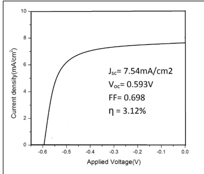
Figure 2.2. Current density versus voltage curve of thin film of ZnO/NG nanocomposite
