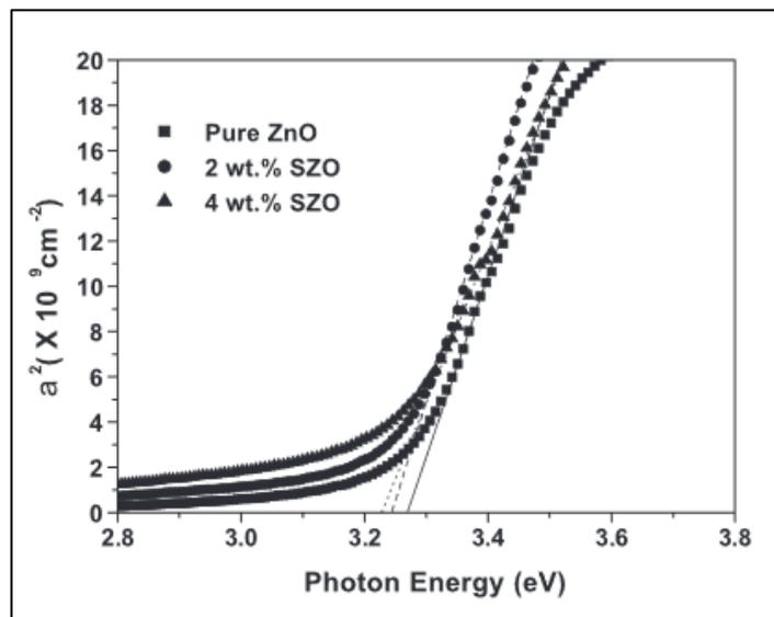
Figure 2.3. The optical band gap of ZnO and SZO at different weight percent.
