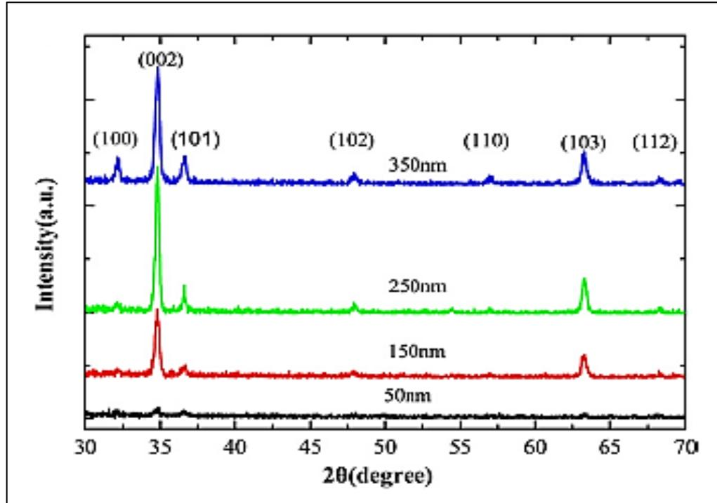
Figure 2.5. XRD patterns of the sol-gel ZnO thin films with different thicknesses annealed at 800 °C
