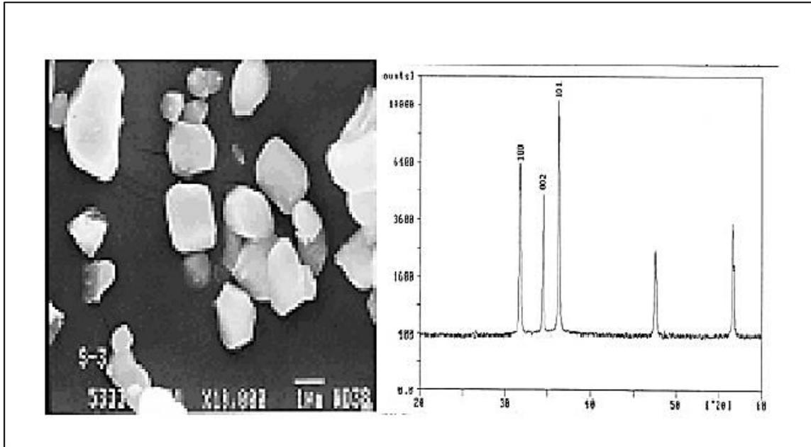
Figure 2.1. SEM and XRD of ZnO bulk crystal
