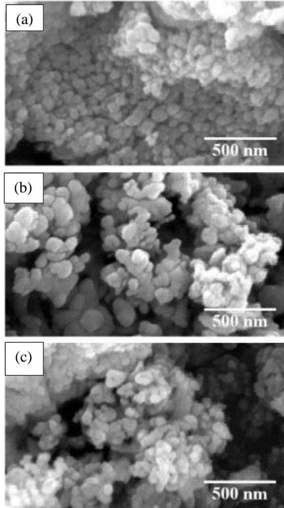
*Figure 2.7.* The FE-SEM morphologies of (a) pure ZnO, (b) 2 % and (c) 7 % Ag doped ZnO nanoparticles.
