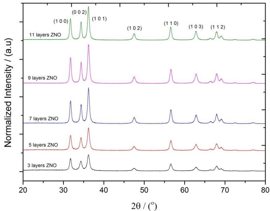
Figure 4.1 (a). XRD spectra of ZnO at 3, 5, 7, 9 and 11 layers
