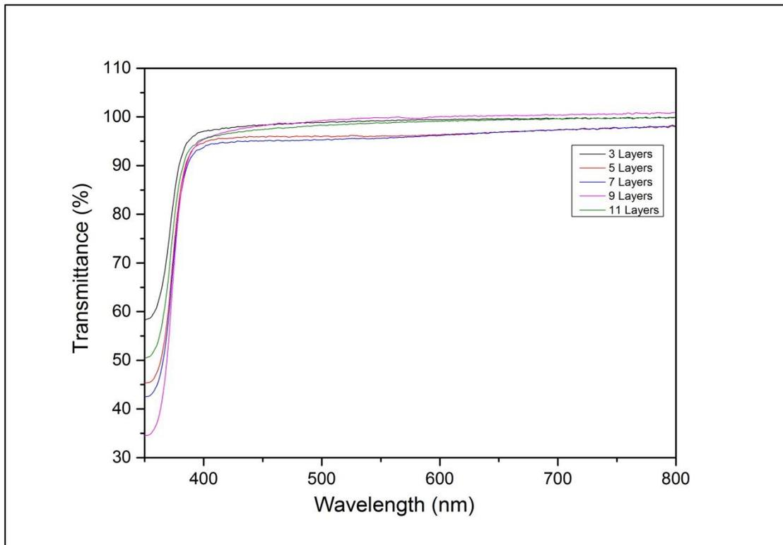
Figure 4.2 (b). UV-visible transmittance spectrum of SZO thin films of 5 different layers
