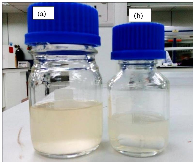
*Figure 3.3.* (a) Pure ZnO (b) Ag-doped ZnO
