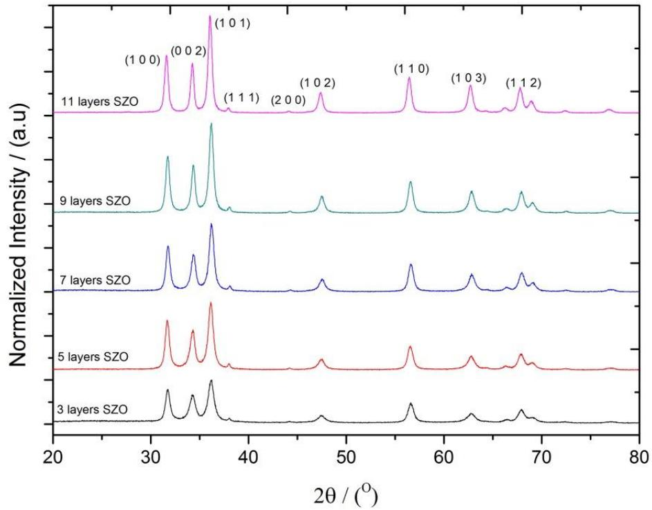
Figure 4.1 (b): XRD spectra of SZO at 3, 5, 7, 9 and 11 layers
