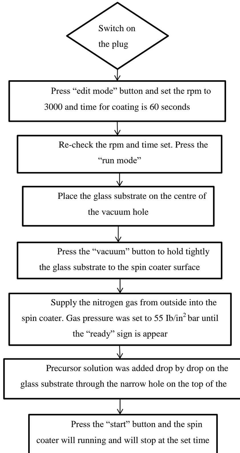
Figure 3.5. Standard operating procedure of spin coating
