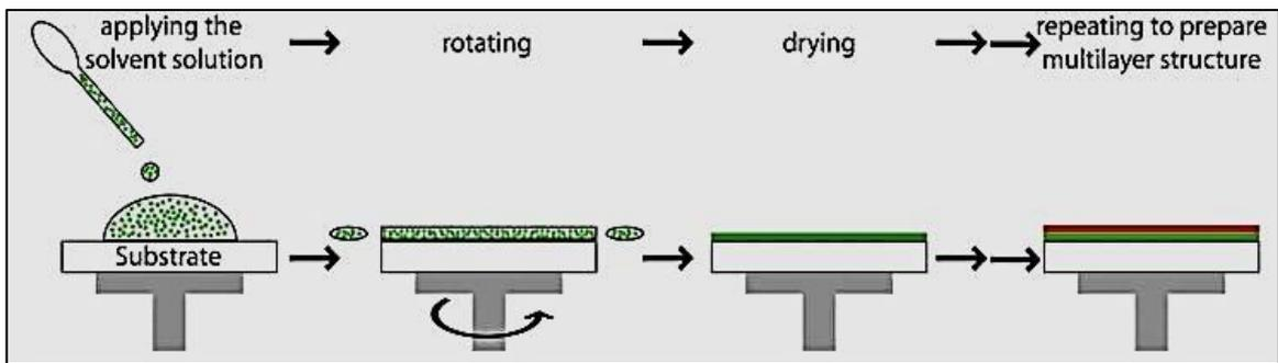
Figure 2.4. Schematic of the spin-coating process
