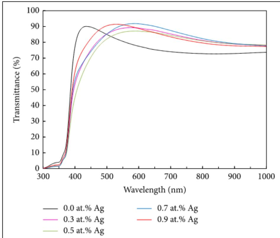
Figure 2.6. UV-Vis transmittance spectra of ZnO and SZO thin films
