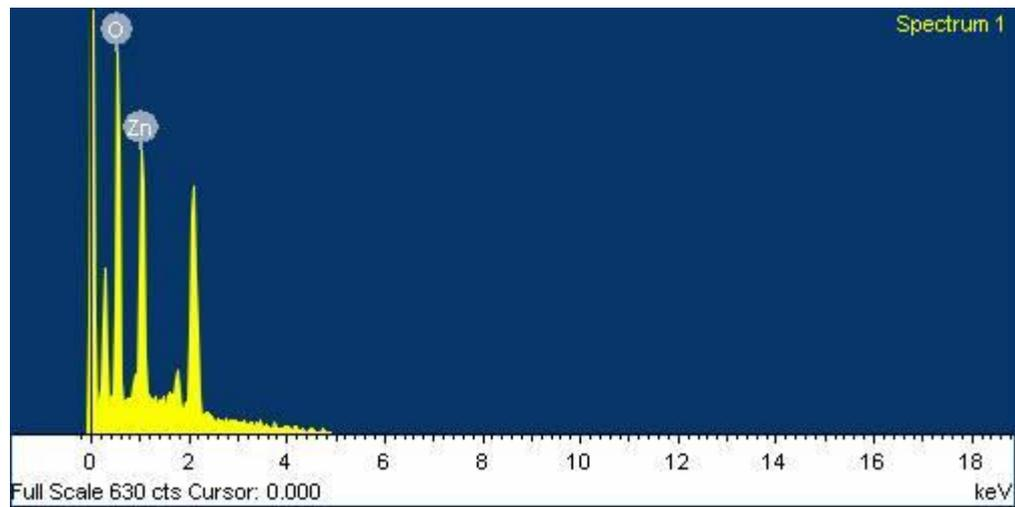
Figure 4.4 (a). EDX pattern of ZnO thin film
