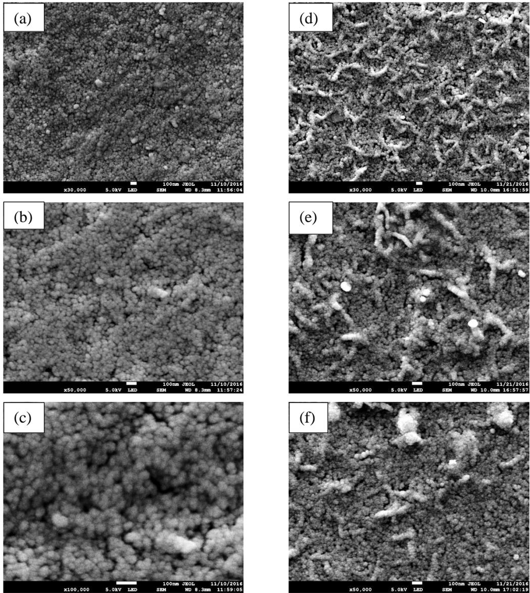
*Figure 4.3.* (a) to (c) FESEM micrograph of ZnO at 3 layers and (d) to (e) SZO at 11 layers.
