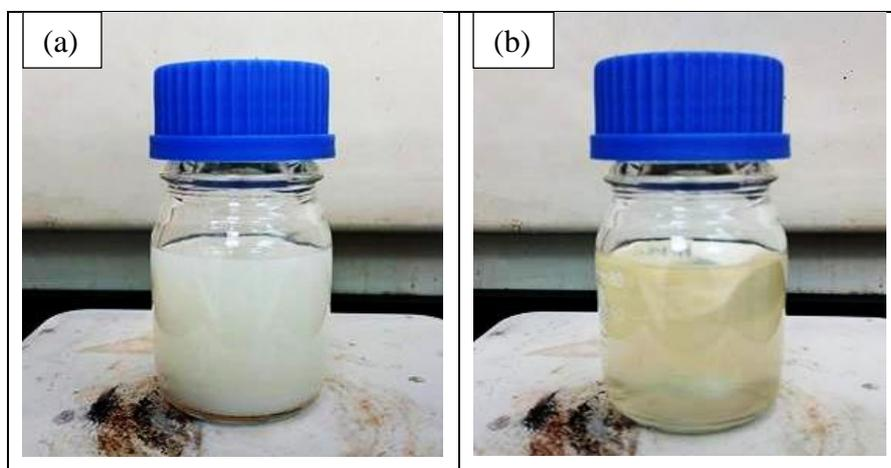
*Figure 3.2.* (a) ZnO solution without DEA while (b) ZnO solution with DEA
