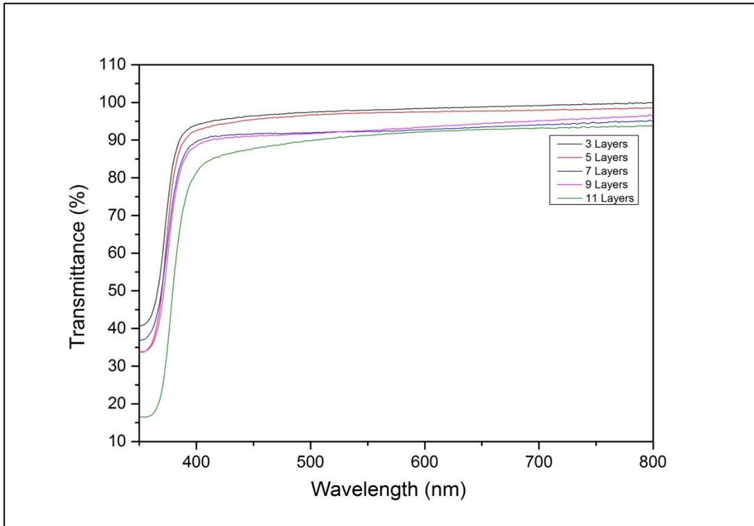
Figure 4.2 (a). UV-visible transmittance spectrum of pure ZnO thin films of 5 different layers
