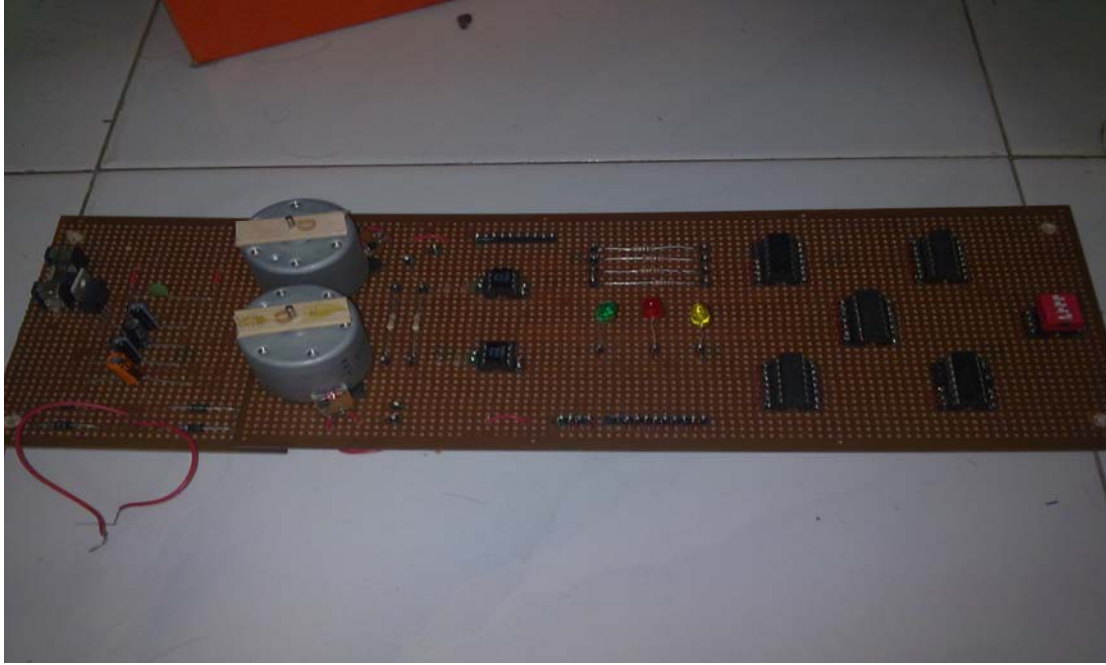
Appendix A.1: Front view of a complete dc ac motor controller switching
