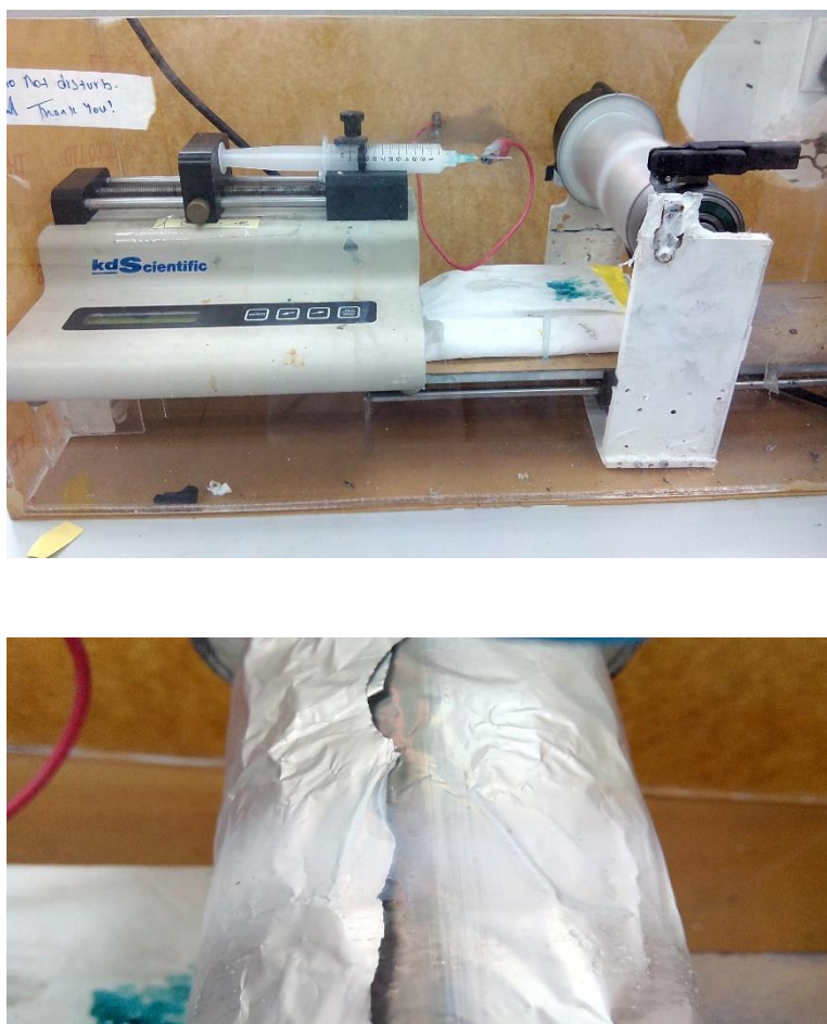
Figure 3.2: The fabrication of PVA/starch using electrospinning technique.
