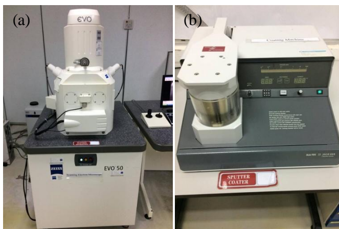
Figure 3. 5. FESEM instrument (a) Zeiss EVO 50 SEM and (b) Baltec-SCD 005 Sputter Coater
